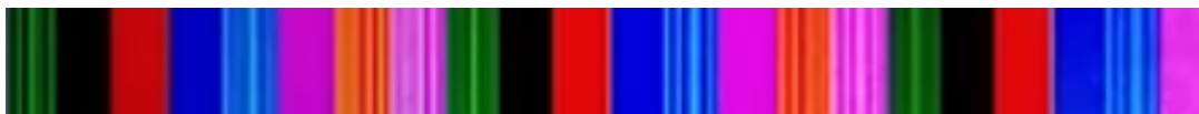
Figure 8.5: The 8-CSK modulation symbols combined with a 20 kHz PWM on the green channel only.
