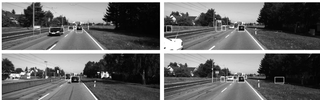
Figure 3.12: Some Detections Results Obtained from KITTI Dataset
