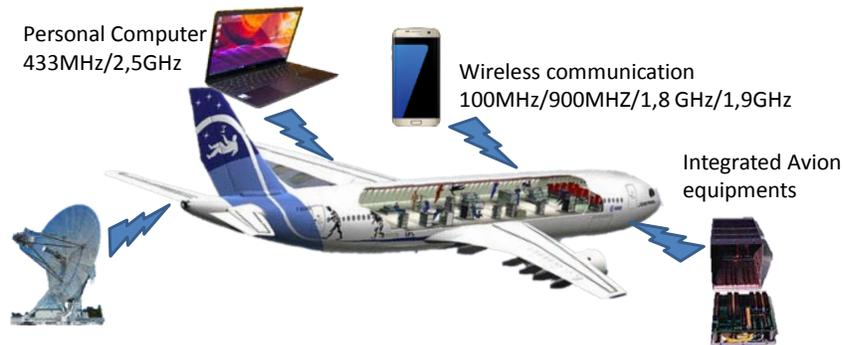
**Figure I-6 Sources of EME in an aeronautical system**
