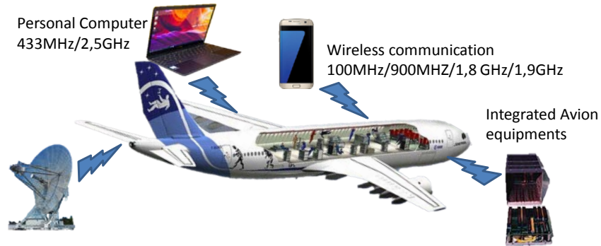
Figure I-6 Sources of EME in an aeronautical system
