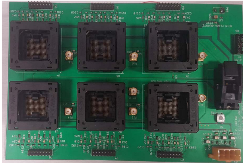
Figure IV-7 Designed PCB for burn-in tests for several FPGAs
