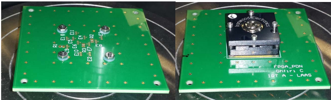
Figure II-16 test board for PDN extraction: bottom side (left), top side (right)
