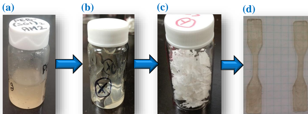
Ph. 1. (a) Synthesized telechelic poly(ethylene- stat -butylene) difunctional initiator terminated by SG1 groups (PEB-(SG1) 2 ), (b) P( My )-(SG1) 2 macro-initiator obtained from My NMP initiated by PEB-(SG1) 2 , (c) dry S- My -S triblock copolymer (sample S 16 - My -S 16 ) obtained via the S chain-extension from P( My )-(SG1) 2 macro-initiator and (d) dog-bone tensile bar specimens (ASTM D638, type V) from sample S 16 - My -S 16 shaped by hot press.
