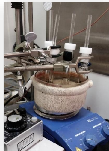
Ph. 1. Polymerization of isoprene using four capacity pressure tubes placed in an oil bath.
