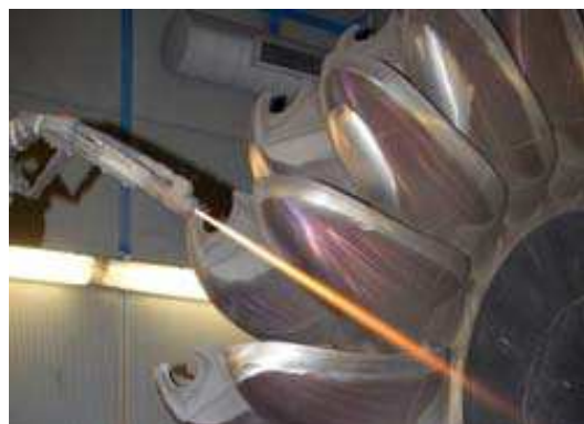
Figure 1.31: HVOF coating on Pelton buckets. ANDRITZ Hydro.
