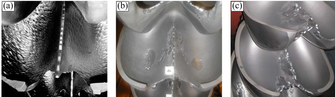
Figure 1.35: Eroded surfaces of Pelton runner without coating and with SHX TM coating after operation : (a) Uncoated Pelton runner after 38,000 t (Alfalfal, Chile), (b) SXH TM 70 after 120,000 t (Alfalfal, Chile), (c) SXH TM 8X after 183,000 t (Alfalfal, Chile). ANDRITZ Hydro.
