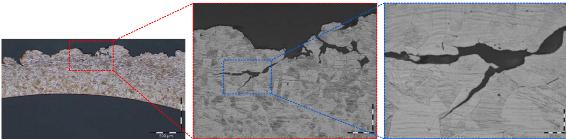
Figure 1.21: Fatigue defects observed on H300 after 5 million (on left) and 10 million (on right) impacts, at impact velocity V = 225 \text{ m.s}^{-1} [LUI 13].
