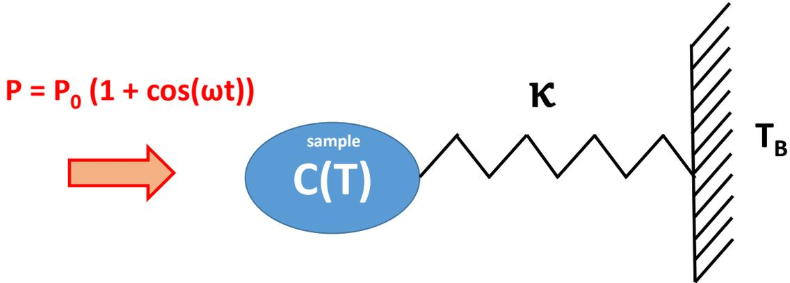
Figure 2.18: **Principle of AC-calorimetry.** The sample is coupled to a thermal bath at the temperature  $T_B$  via the thermal coupling  $\kappa$  and is heated by an alternating power  $P = P_0(1 + \cos(\omega t))$ .
