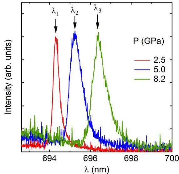
Figure 2.17: **Ruby fluorescence.** Measured ruby spectra at 4 K for different values of the pressure. One can see that the R-line peak shifts to higher values of  $\lambda$  with increasing the pressure.
