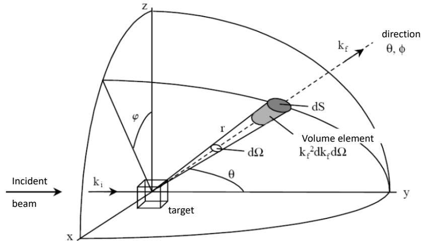
Figure 2.2: **Sketch of a scattering process by a "target".**  $k_i$  and  $k_f$  denote the initial (incident) and the final (scattered) wave-vector respectively. The scattered beam is indicated by the angles  $\phi$  and  $\theta$ . Figure taken from [Son16; Gre11].
