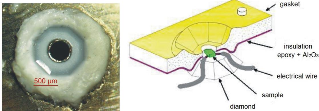
Figure 2.15: **Elaboration of the gasket.** Left: gasket with the insulating mixture. One can see the hole at the center of the gasket and the imprint of the diamond anvils. Right: Scheme of the setup of a DAC cell with the gasket, the wires, the sample and the anvils. Figure extracted from [Fer12].
