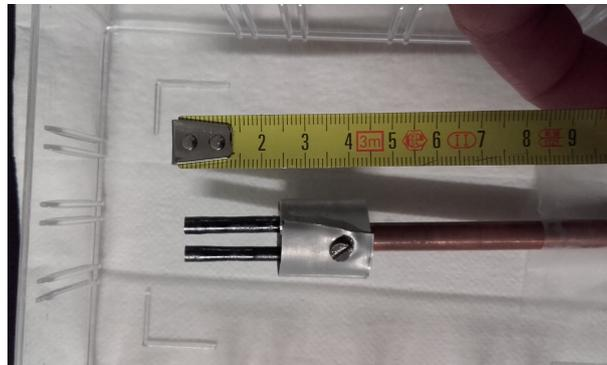
Figure 5.7: **Photograph of the two co-aligned  $\text{BaCo}_2\text{V}_2\text{O}_8$  single crystals.** The two crystals were glued on a copper sample holder with black stykast to ensure a good thermal contact. A ring of Cadmium was added to avoid the scattering noise from the glue.
