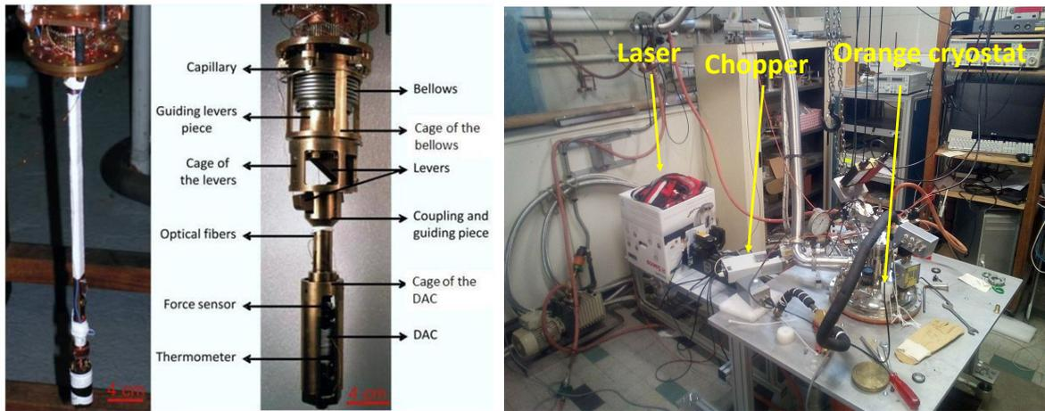
Figure 6.2: **Experimental setup of specific heat measurements under high pressure, magnetic field and low-temperature.** Left: The stick of the orange cryostat where the DAC is inserted. The stick is equipped of levers which allow to apply a force (and thus a pressure) on the DAC. Right: Picture of the experimental setup. The stick is now inside the orange cryostat which is surrounded by a magnetic coil. The laser and the chopper are also shown.
