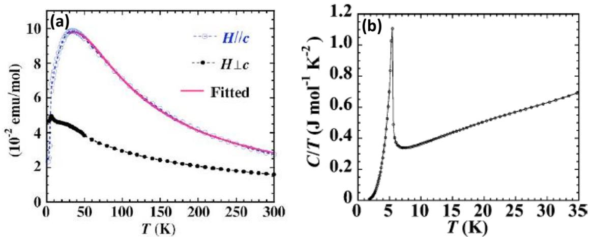
Figure 1.15: **Macroscopic characterization of the magnetic properties of  $\text{BaCo}_2\text{V}_2\text{O}_8$ .** (a) Susceptibility  $\chi$  as a function of  $T$  for two different orientations of the magnetic field set to  $\mu_0 H = 1$  T. (b) Temperature dependence of the specific heat at zero-field. Figures extracted from [He+05a; He+05b].
