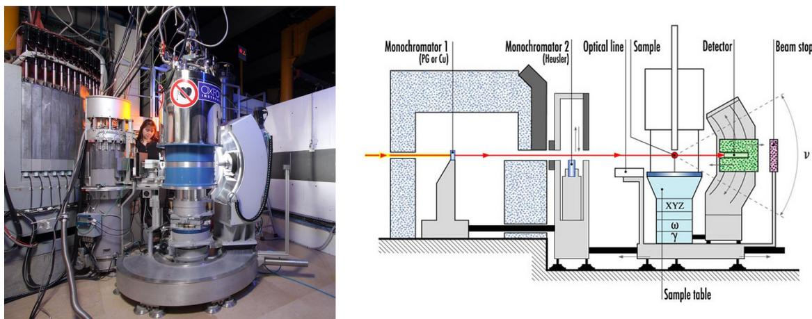
Figure 2.10: **2-axis diffractometer D23 at ILL.** Left: picture of the diffractometer with a 12 T vertical cryomagnet. Right: Sketch of the instrument with the different angles:  $\omega$  for the rotation of the sample and  $(\gamma, \nu)$  for the lifting-detector position. Figure extracted from [D23].
