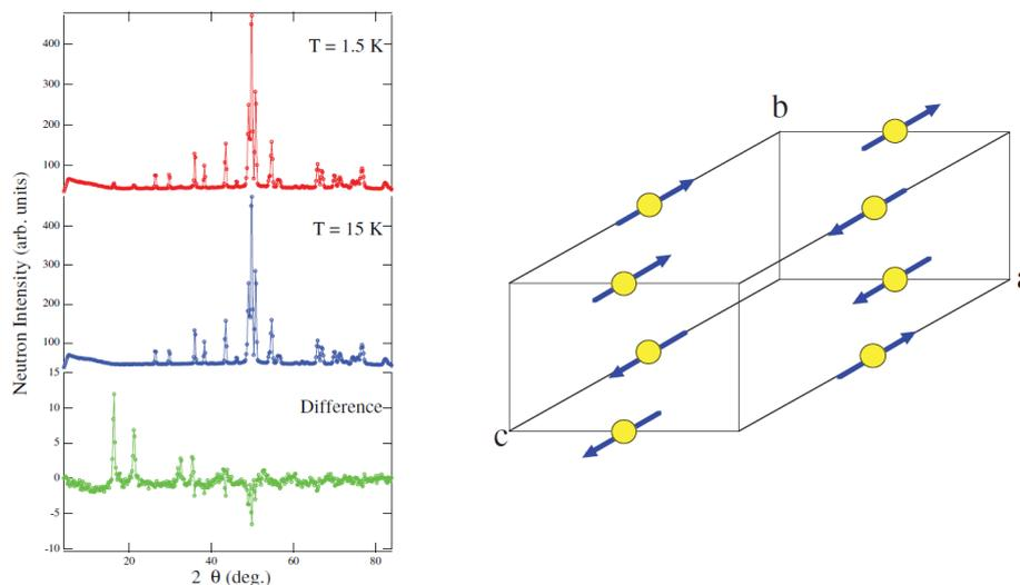
Figure 2.8: **Example of the determination of a magnetic structure.** Left: Powder diffraction patterns recorded below and above the transition temperature in the compound  $\text{Cr}[\text{C}(\text{CN})_3]_2$  and difference. Right: Schematic representation of the magnetic structure of  $\text{Cr}[\text{C}(\text{CN})_3]_2$  at 2K. For sake of clarity, only the Cr atoms of the unit cell have been represented. Figures extracted from [MRM00]
