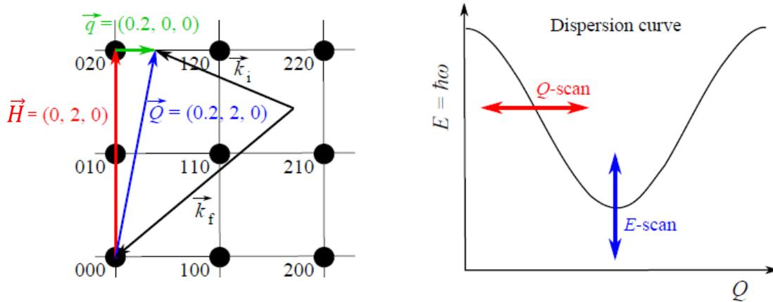
Figure 2.12: **Principle of an inelastic neutron scattering experiment.** Left:  $k_i \neq k_f$  with  $\vec{Q}$  in the horizontal plane ( $a^*$ ,  $b^*$ ).  $\vec{H}$  is a vector of the reciprocal lattice,  $\vec{q}$  is a wave-vector of the Brillouin zone. Right: The two kinds of measurements leading to the dispersion curve  $E = f(Q)$ :  $Q$ -scan at constant energy (in red) and  $E$ -scan at constant scattering vector  $\vec{Q}$  (in blue). Figures extracted from [Can10]
