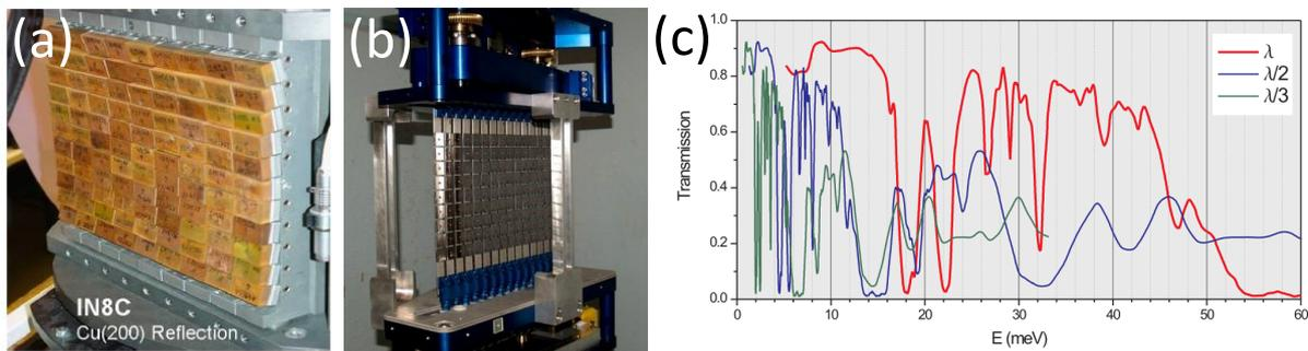
Figure 2.7: **Examples of monochromator:** (a) of copper and (b) of silicon. (c) Graphic showing the transmission of the fundamental wavelength  $\lambda$  and its two first harmonics  $\lambda/2$  and  $\lambda/3$  by a Pyrolytic Graphite (PG) filter. For  $E = 13.5 \text{ meV}$  ( $\approx 2.46 \text{ \AA}$ ), the two harmonics are suppressed. Figure extracted from [ETH].
