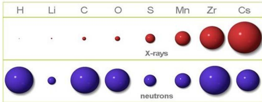
Figure 2.3: **Difference between neutrons and X-rays cross sections.** The cross section of the X-rays is increasing with the size of the atom, i.e. its number of electrons and thus its atomic number  $Z$ :  $\sigma_{\text{X-rays}} \propto Z^2$ . For the neutrons, we have  $\sigma_{\text{neutrons}} \propto b^2$  with  $b$  the scattering length which varies randomly from one atom to another. In particular, neutrons are very sensitive to hydrogen while X-rays are not.
