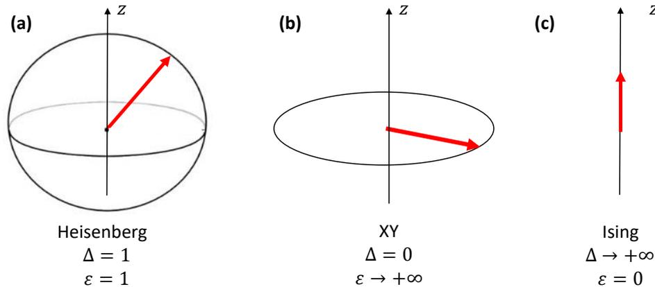
Figure 1.8: **Different anisotropies.** The red arrow indicates one orientation of the spin among all the possible ones (shown by the black sphere, circle or line). (a) Heisenberg case where the orientation of the spin is isotropic. (b) XY case where the spin lies in the plane perpendicular to  $z$ . (c) Ising case where the spin points along the  $z$  direction.
