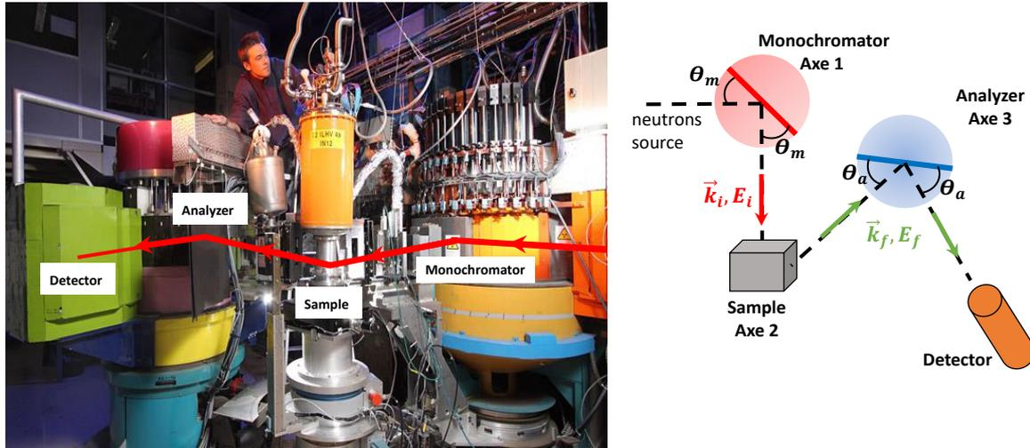
Figure 2.13: **Three-axis-spectrometer.** Left: Picture of the 3-axis spectrometer IN12 at ILL. Figure extracted from [IN1]. Right: Sketch of the principle of a triple-axis spectrometer from a top view.
