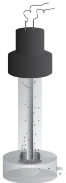
Figure 1.30: Dead-end stirred cell for membrane emulsification commercialised by Micropore Technologies [65]
