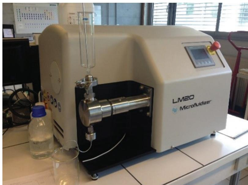
Figure 2.18: Photography of the Microfluidizer processor
