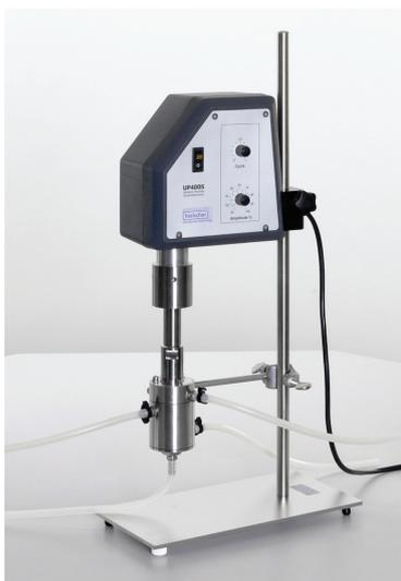
Figure 2.17: Photography of an UP400S Ultrasonic Processor
