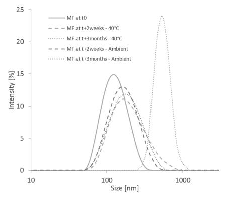
Figure 6.12: Comparison of size distributions in intensity (DLS) at t0, t+2 weeks and t+3months for different stability conditions, ambient temperature and  $40^{o}$ C for MF sample at cycle 5
