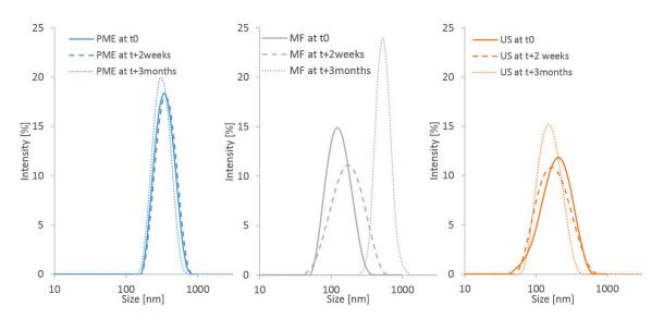
Figure 6.7: Comparison of size distributions in intensity (DLS) at t0, t+2 weeks and t+3months under accelerated stability at  $(40^{o}\text{C})$  for nanoemulsions prepared by PME, MF and US with selected conditions
