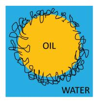
Figure 1.5: Droplet stabilization by steric hindrance
