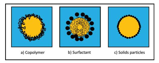
Figure 1.9: Different types of molecules showing a surface activity and stabilizing emulsions
