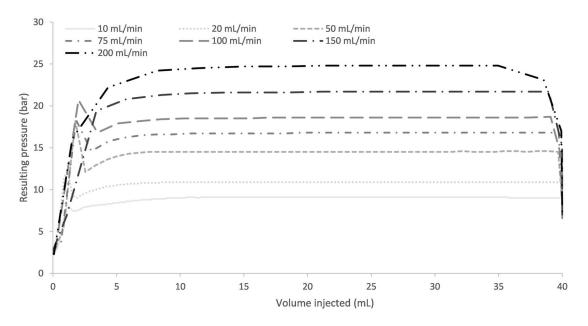
Figure 3.3: Pressure profiles at different flowrates with a 125 mm length and 0.5  $\mu$ m pore size membrane at a composition of 10% EHP and 5% overall surfactant concentration
