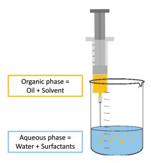
Figure 1.12: Schematic representation of nanoprecipitation set-up
