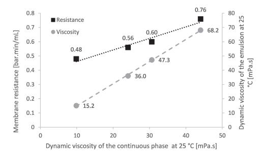
Figure 4.11: Membrane resistance variation with flowrate and dynamic viscosity of the emulsion as a function of continuous phase viscosity
