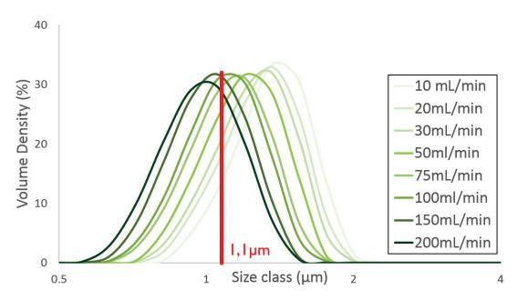
Figure A.6: Size distribution in volume for different flowrates with 1.1  $\mu m$  membrane 10% EHP and 5% surfactant
