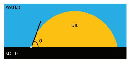
Figure 1.2: Oil/Water/Solid Interface and contact angle (θ)
