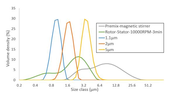
Figure A.4: Size distribution in volume for different membrane pore sizes at 200 mL/min, 10% EHP and 5% surfactants
