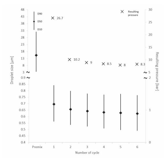
Figure 3.7: Droplet size and pressure variation with cycle number with 125 mm length and 0.5  $\mu$ m pore size membrane at 200 mL/min at a composition of 10% EHP and 5% overall surfactant concentration
