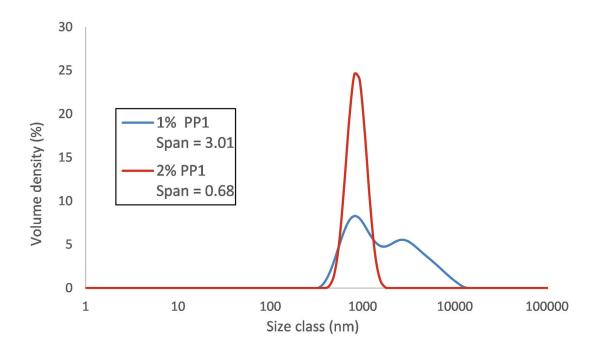
Figure 5.2: Size distribution in volume at different polypeptide concentrations and 10% oil with the 0.8  $\mu m$  membrane
