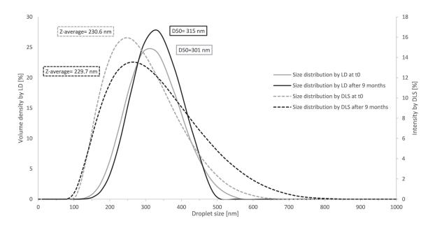
Figure 3.11: Example of nanoemulsion stability observed at 9 months for nanoemulsion obtained with a 125 mm length and 0.2  $\mu$ m pore size membrane at 5 mL/min
