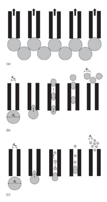
Figure 1.34: Droplet break-up in PME from [62] (a) Droplet retention under a critical pressure, (b) Moderate break-up at moderate shear stress, (c) Intensive break-up at high shear stress
