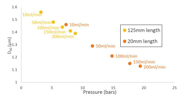
Figure A.5: Influence of membrane length on resulting pressure and size with 1.1  $\mu m$  membrane at 10% EHP and 5% surfactants
