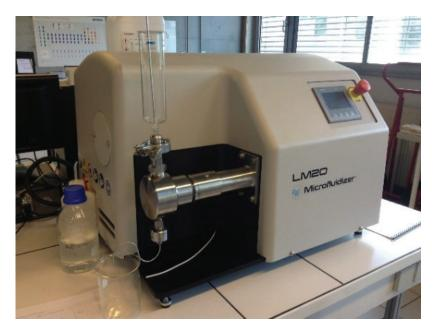
Figure 2.18: Photography of the Microfluidizer processor
