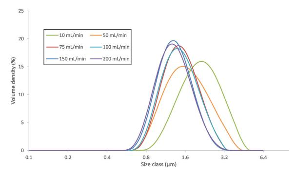
Figure 5.4: Size distribution in volume for different flowrates with the 1.1  $\mu m$  membrane at 10% oil and 2% PP1
