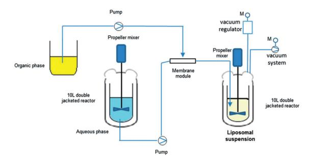
Figure 1.32: Large scale set-up for liposomes production [71]
