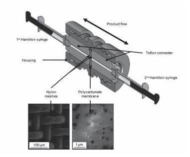
Figure 1.31: Schematic representation of an extruder device for liposomes homogenization or nanoemulsion production [59]
