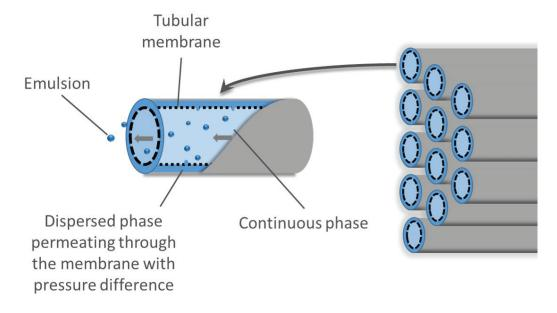
Figure 1.21: Schematic figure of direct membrane process principle
