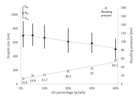
Figure 3.8: Droplet size and pressure variation as a function of oil weight percentage in the formulation with 125 mm length and 0.5  $\mu$ m pore size membrane at 150 mL/min
