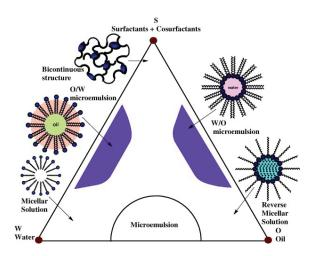
Figure 1.13: Schematic microemulsion domain in a phase diagram from Malik et al. [30]
