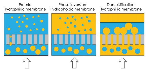
Figure 1.23: Different types of utilization of PME
