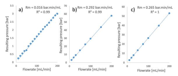
Figure 2.14: Examples of different Rm measured a) 125 mm long membrane with 0.5  $\mu$ m pore size b) 20 mm long membrane with 0.3  $\mu$ m pore size c) 125 mm long membrane with 0.1  $\mu$ m pore size
