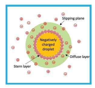
Figure 1.4: Electrical double layer of a charged emulsion
