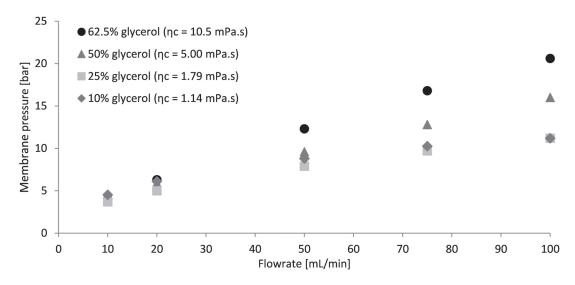
Figure 4.4: Membrane pressure variation with flowrate from 10 to 100 mL/min at four different concentrations in glycerol in the water phase and at 10 % of Marcol 82 and 5% surfactant
