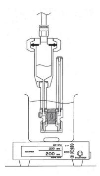
Figure 1.28: External pressure type microkit available at SPG Technology Co., Ltd, schematic view from the supplier brochure
