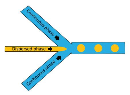
Figure 1.15: Schematic representation of a microfluidic device
