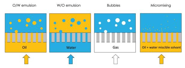
Figure 1.22: Different type of formulation that can be produced with DME
