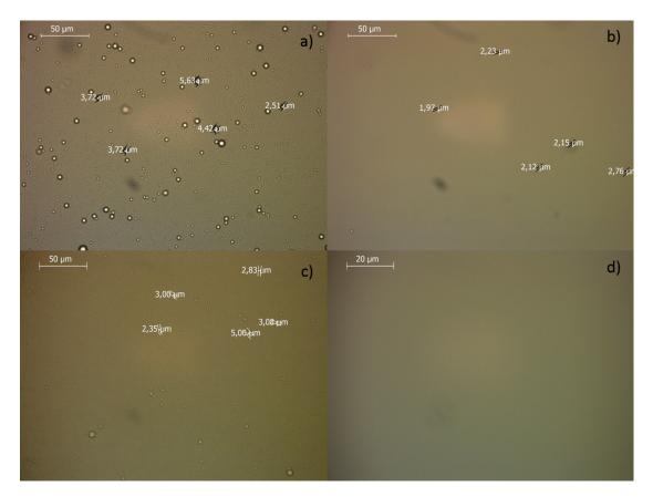
Figure 6.6: Optical microscopy photographs at x40 of three emulsions a) first cycle of MF at 1000 bars; b) fifth cycle of MF at 1000 bars; c) 5 min at 60% intensity US; and one at x 100, d) fourth cycle of PME
