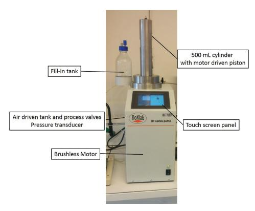
Figure 2.4: Photography of the high pressure syringe pump
