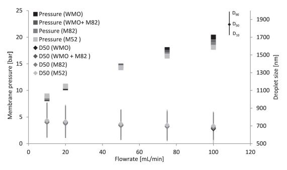
Figure 4.6: Membrane pressure and droplet size at different flowrates with different oils or oil mix at 10% and 5% overall surfactant concentration
