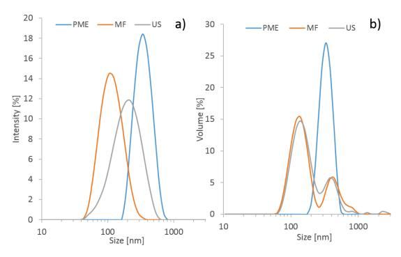
Figure 6.5: Comparison of size distribution in intensity by DLS a) and in volume by LD b) for the three different processes PME,MF and US for selected conditions
