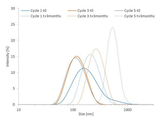
Figure 6.11: Comparison of size distributions in intensity (DLS) at t0 and t+3months accelerated stability at  $40^{o}$ C for the different cycle number in MF
