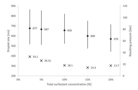
Figure 3.10: Evolution of droplet size and resulting pressure with total surfactant concentration with 125 mm length and 0.5  $\mu$ m pore size membrane at 200 mL/min at 10% EHP concentration
