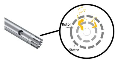
Figure 1.14: Principle of rotor stator systems
