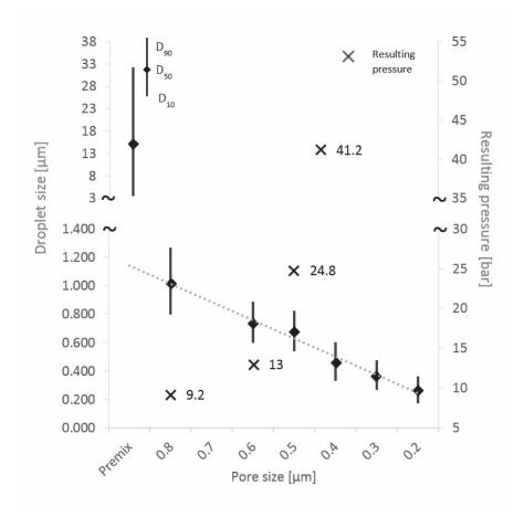
Figure 3.5: Droplet size distribution of the premix and nanoemulsions obtained at different pore sizes (at 200 mL/min, except for 0.3  $\mu$ m pore size membrane at 100 mL/min and 0.2  $\mu$ m pore size membrane at 5mL/min) and resulting pressure except for 0.2  $\mu$ m and 0.3  $\mu$ m pore size membrane as flowrate was changed, at a composition of 10% EHP and 5% overall surfactant concentration
