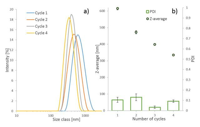
Figure 6.2: Effect of cycles number on particle size distribution in intensity a); Z-average and PDI b) by DLS for PME at cycles 1 to 4
