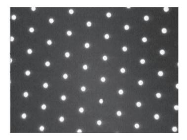
Figure 1.26: Optical microscopy photography of a 30  $\mu m$  regular pore size micro-engineered metallic membrane (Micropore Technologies Ltd)[54]
