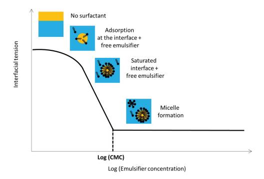
Figure 1.8: Evolution of the interfacial tension with emulsifier concentration and oil, water and emulsifier interactions
