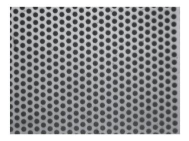
Figure 1.27: Optical microscopy photography of a silicon micro-engineered membrane with an uniform 5  $\mu$ m pore size and a porosity of 30% [55]
