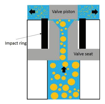
Figure 1.16: Schematic representation of a high pressure homogenizer
