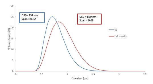
Figure 5.5: Size distributions for the smallest emulsion obtained with PP2 at 2%,  $0.8\,\mu m$  membrane and 10% oil just after production, (t0) and after 9 months at room temperature (t+9 months)
