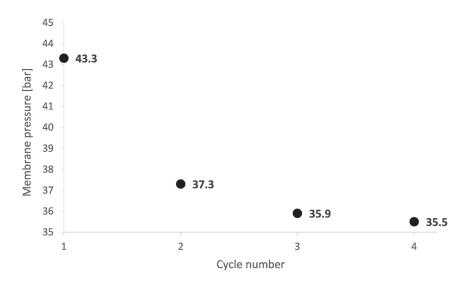
Figure 4.14: Effect of cylcle number on membrane pressure at a composition of 10% water, 5% surfactant and 85% Marcol 82 at a flowrate of 50 mL/min
