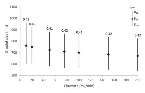
Figure 3.4: Droplet size as function of flow rate with a 125 mm length and 0.5  $\mu$ m pore size membrane at a composition of 10% EHP and 5% overall surfactant concentration
