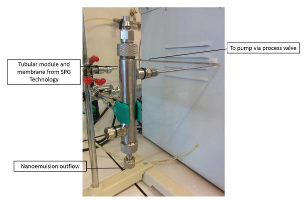
Figure 2.3: Connection of the cross-flow tubular module to the high pressure syringe pump
