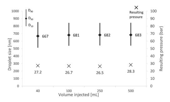
Figure 3.2: Resulting pressure and droplet size variation with scaling up from 40 mL to 500 mL with 125 mm length and 0.5  $\mu$ m pore size membrane at 200 mL/min at a composition of 10% EHP and 5% overall surfactant concentration
