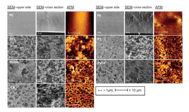
Figure 1.25: SEM and AFM photographies of seven different types of polymeric membranes [53] PC: polycarbonate; PES: polyethersulfone; CA: cellulose acetate; PE: polyester; PS: polysulfone; PVDF: polyvinylidene fluoride
