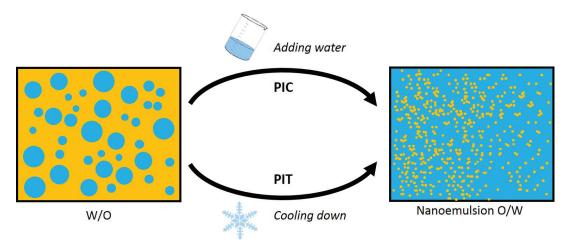
Figure 1.11: Schematic representation of phase inversion methods
