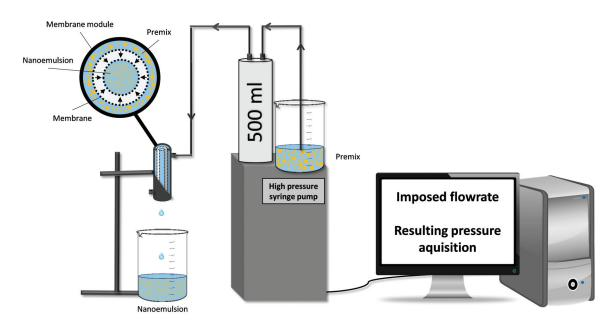
Figure 2.2: Schematic representation of the experimental set-up
