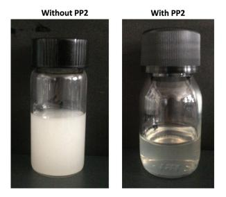
Figure 5.9: Composition: dispersed phase 10 % of a 30/70 citrate buffer /glycerol mixture with or without 1 % PP2; continuous phase: 90 % of 20 % Ewocream in MCT oil
