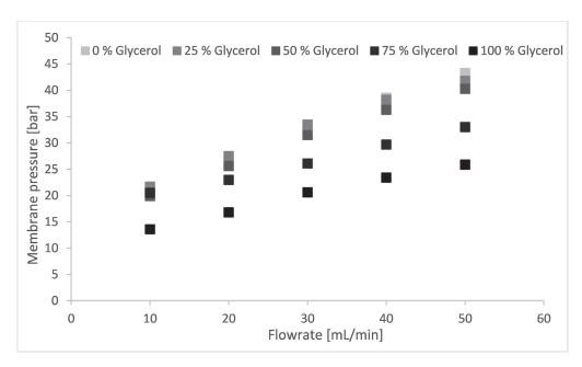
Figure 4.12: Variation of membrane pressure for different amounts of glycerol in the dispersed phase, with oil and surfactant content kept constant at 10% and 5% respectively
