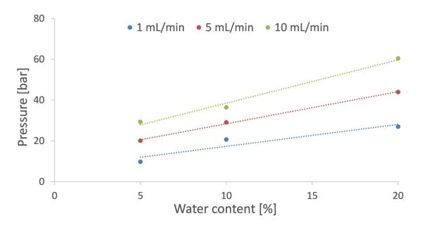
Figure 5.7: Variation of the resulting pressure with water phase content at various flowrates
