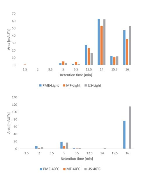
Figure 6.9: Peak areas at different retention times after 2 weeks in stability at day light exposure and  $40^o\mathrm{C}$
