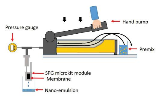
Figure 2.1: Schematic representation of the proof of concept set-up
