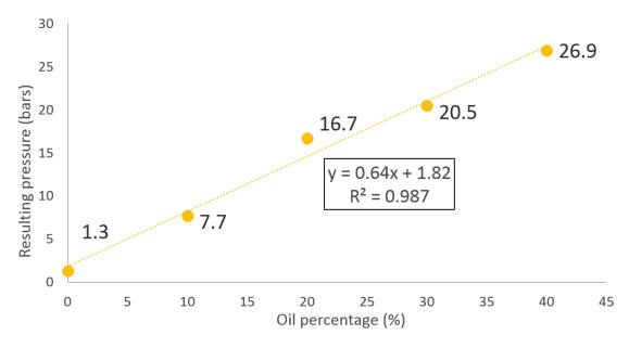
Figure A.7: Resulting pressure variation with oil concentration at a surfactant/oil ratio of 10% with  $1.1\,\mu m$  membrane
