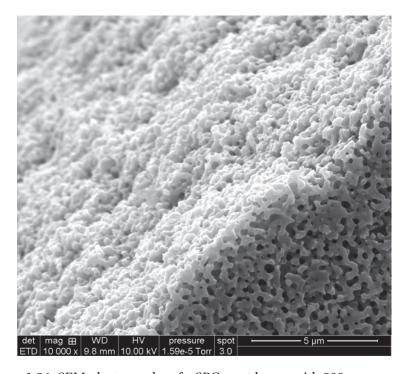
Figure 1.24: SEM photography of a SPG membrane with 200 nm pore size
