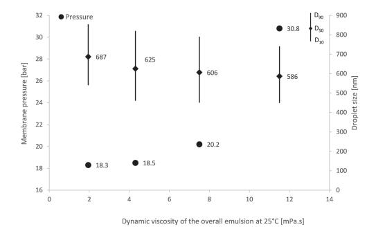
Figure 4.7: Membrane pressure and droplet size as a function of dynamic emulsion viscosity for different oil contents at 100 mL/min
