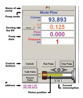
Figure 2.5: Details of the control panel
