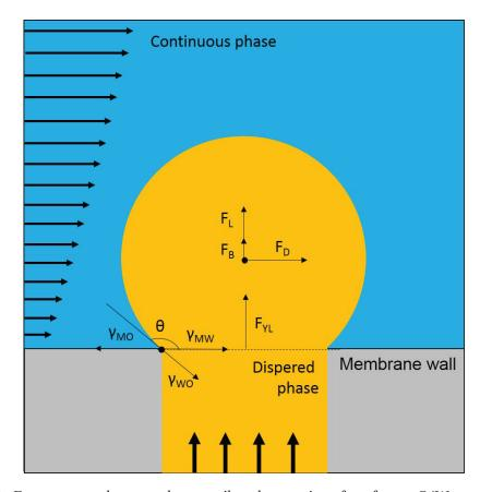
Figure 1.33: Forces exerted at membrane, oil and water interface for an  ${\rm O/W}$  emulsion and an hydrophillic membrane
