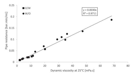
Figure 4.3: Slope of the resulting pressure,  $\Delta P_{pipe}$  with flow rate as a function of viscosity for O/W and W/O emulsions of different composition
