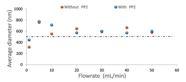
Figure 5.10: Variation of the average droplet diameter as a function of flowrate for emulsions with or without PP2. Emulsification conditions: membrane pore size  $0.5 \mu m$
