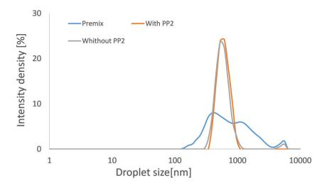
Figure 5.8: Size distribution comparison of the emulsions obtained with or without PP2 after passing through a 0.5  $\mu$ m pore size membrane at a flowrate of 30 mL/min. Composition: dispersed phase 10 % of a 30/70 citrate buffer /glycerol mixture with or without 1 % PP2; continuous phase: 90 % of 20 % Ewocream in MCT oil
