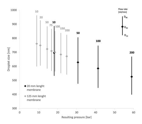
Figure 3.6: Droplet size as a function of resulting pressure for different membrane length and different flowrates with a 0.5  $\mu$ m pore size membrane at a composition of 10% EHP and 5% overall surfactant concentration
