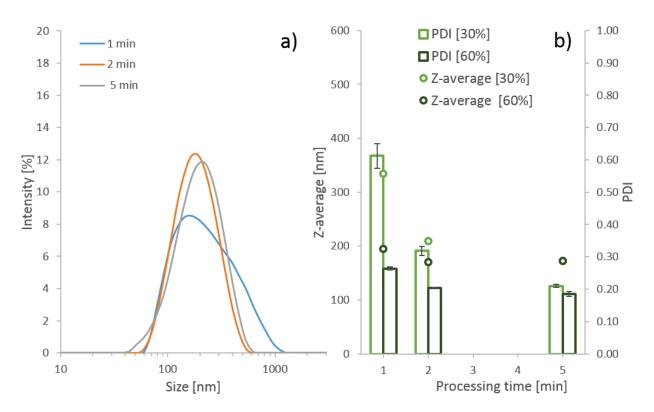
Figure 6.4: Effect of US duration from 1 min to 5 min on particle size distribution in intensity by DLS a) and effect of US duration and intensity on Z-average and PDI b)
