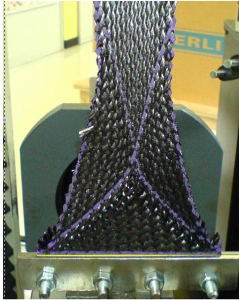
Figure 9: Shear behavior in the plane of the yarns of fibrous composite reinforcements.
