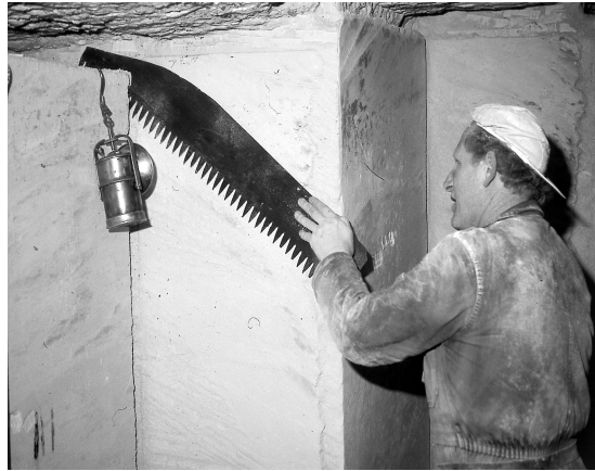
Figure 3.1: Miner in a underground quarry, using a special handsaw to cut a Tuffeau de Maastricht block from the surrounding rock, after Dubelaar et al. (2006).
