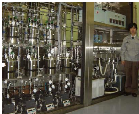
Figure 13 Industrial pilot plant (10 t/year ) with three micro-reactor blocks for radical polymerisation in Japan 8
