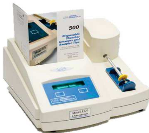
Figure 3-6. The advance micro-osmometer is the standard system for the determination of the total osmolality in aqueous solutions using the freezing point depression. It necessitates 20 µl of samples.
