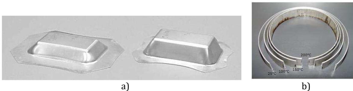
Figure 1.6 – Advantages of warm forming: a) formability increase (Bolt et al., 2001); b) springback decrease (Grèze et al., 2010)
