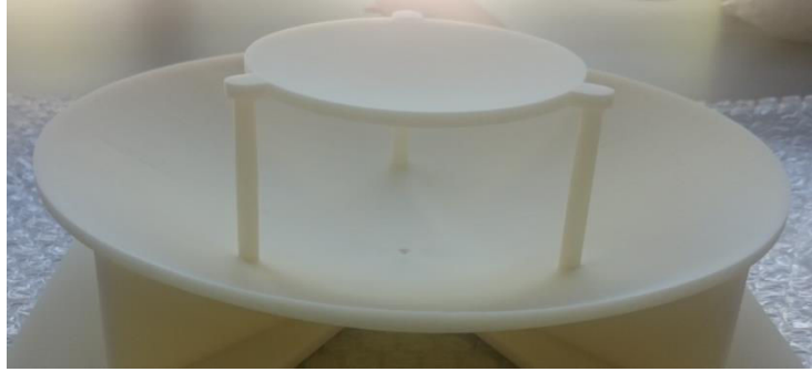
Figure III.66. Prototyped Cassegrain antenna (without metal surface coating).
