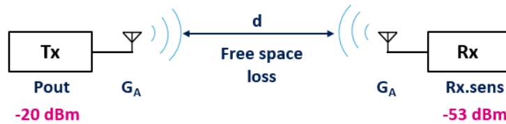
Figure I.32. Schematic of a 240 GHz wireless link based on a Silicon Photonics Tx and a commercial sub-harmonic mixer Rx for link budget estimation.
