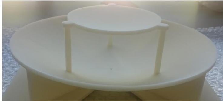
Figure III.66. Prototyped Cassegrain antenna (without metal surface coating).
