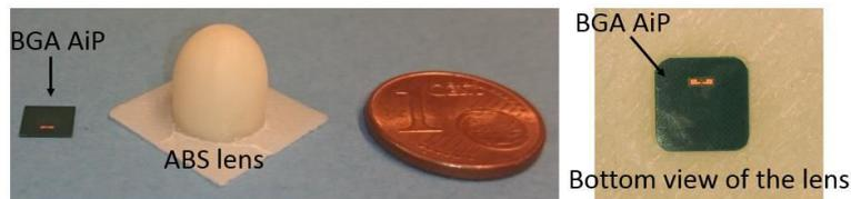
Figure III.60. Picture of prototyped AiP-lens system.
