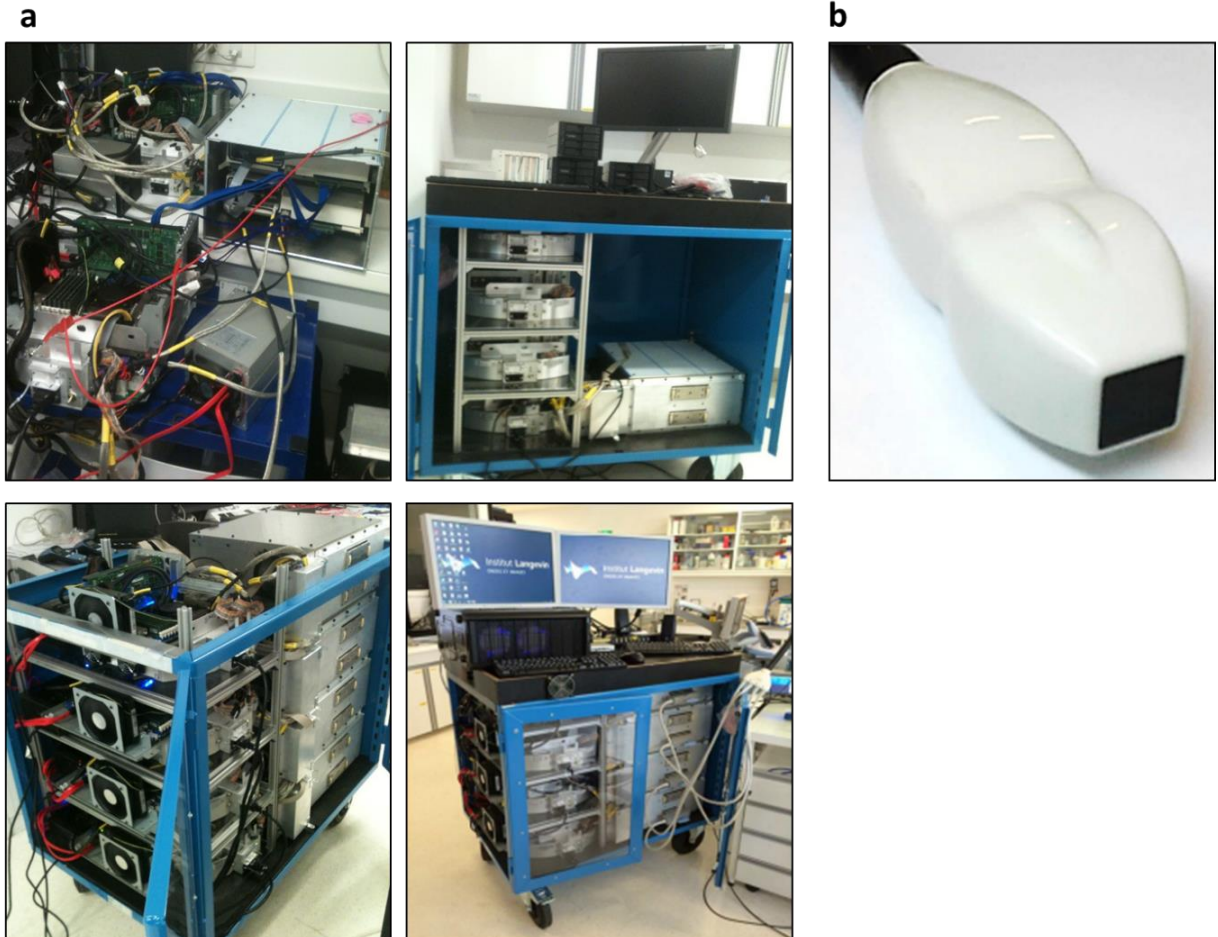
Figure 2.17 – Customized 3D ultrafast ultrasound device. (a) Construction steps of the 3D ultrafast ultrasound scanner. 1024 emitting channels, 512 receiving channels, up to 10 000 volume/s. (b) 2D matrix array, 1024 elements, ( 32 \times 32 ) with 0.3 mm 2 pitch.
