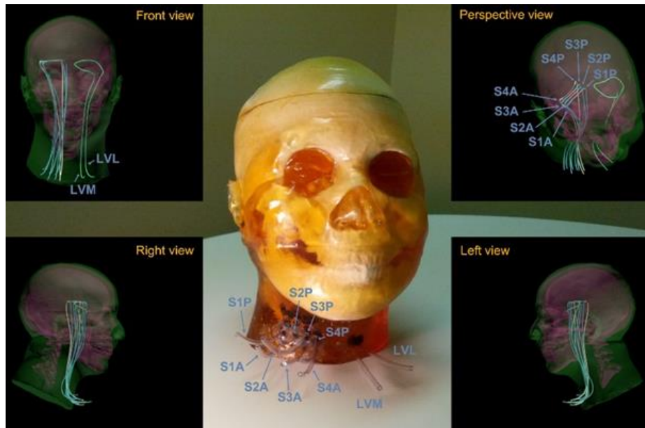
Figure 4.26 – Head phantom developed for transcranial Doppler imaging. Produced by True Phantom Solutions.
