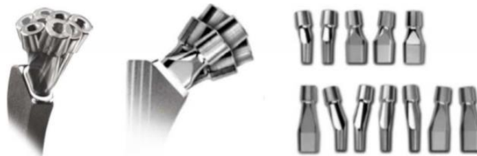
Figure I.2. Types of modular femoral necks (Wright Medical Technology; Arlington TN). Neck types are neutral (135°), varus (127°), valgus (143°), anteverted / retroverted (8° / 15°), or a combination or varus / valgus + anteverted / retroverted [14].
