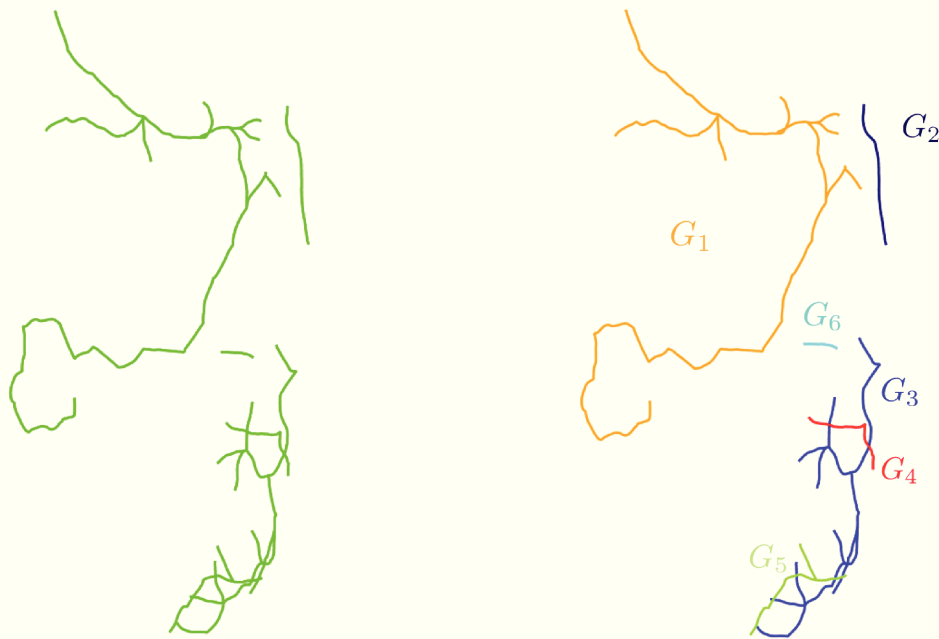
Figure 5.9: Decomposition of selected features into connected sub-graphs of paths that can be processed separately. Left: selected features. Right: each connected sub-graphs of paths is plotted with a particular color.
