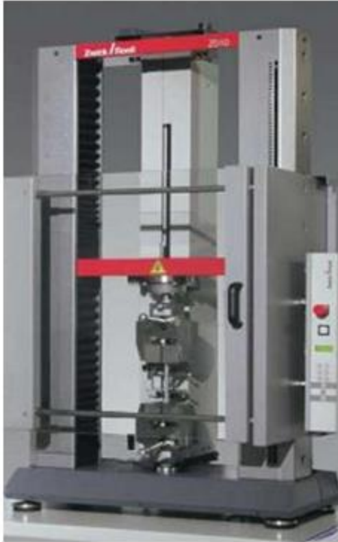
Figure II-3. A universal testing machine for tensile test and the specimen model
