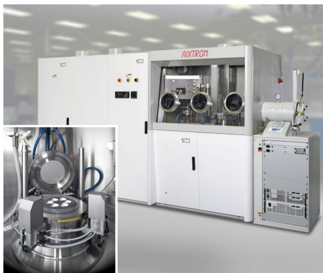
Figure 2.6: A picture of the CCS reactor used in the second part of the thesis. It is possible to notice the gas panel on the left, the glove box and the reactor in the center and the transfer chamber on the right. In the inset, the open reactor (in the 6x2" configuration) is showed.
