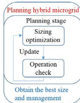
Figure 2.1: Sizing and operation.
