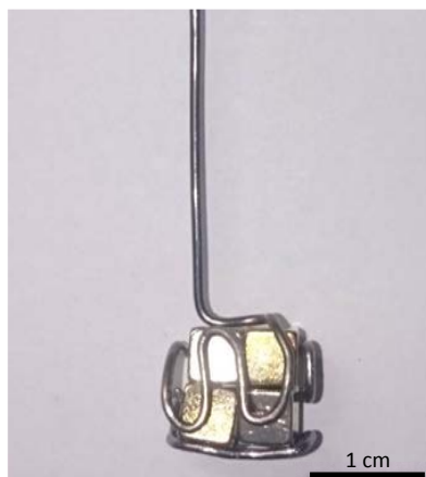
Fig. 80: Picture of the anode configuration before the electrolysis; four magnets are fixed together with a tantalum wire.
