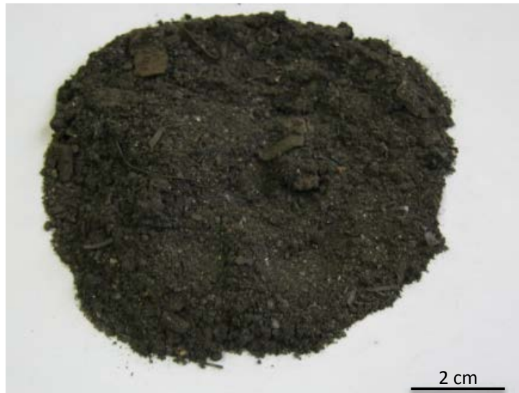
Fig. 77: Picture of the magnetic waste fraction, which was analysed by EDX
