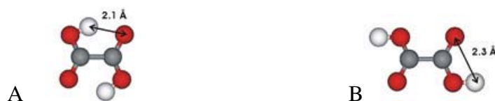
Figure 3.9 Initial geometry of the oxalic acid (a) as modeled in the present MD simulations. Example of the other stable geometry of oxalic acid (b) as taken from ab initio calculations of Mohajeri and Shakerin [118]
