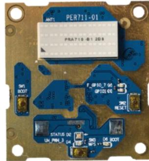
Figure I.19 PERASO X710 long range WiGig array chipset featuring the PRA710 phased array from [I.43].
