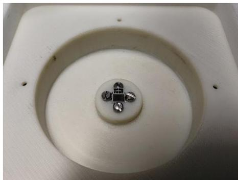
Figure IV.29 Plastic support used to hold the AuT in V-band measurements.
