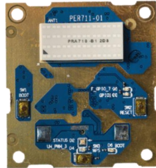
Figure I.19 PERASO X710 long range WiGig array chipset featuring the PRA710 phased array from [I.43].
