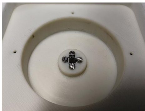
Figure IV.29 Plastic support used to hold the AuT in V-band measurements.
