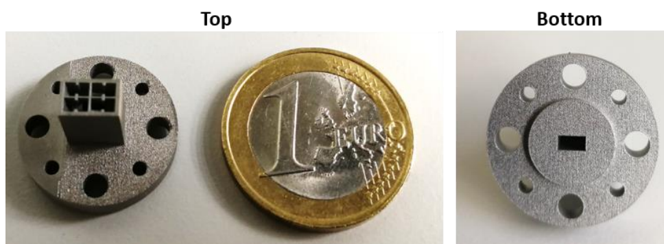
Figure IV.24 Photographs of the 2×2 DRWG 3D printed by micro laser sintering.
