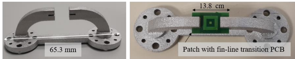
Figure II.43 Pictures of the fabricated samples of the back-to-back waveguide bends with welcome slit for the PCB.
