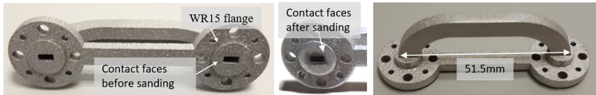
Figure II.42 Pictures of our fabricated samples for the back-to-back waveguide bends.
