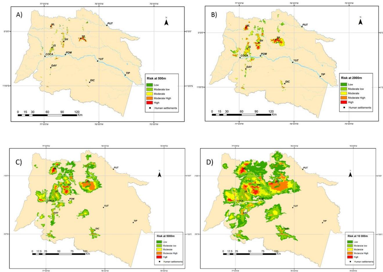
**Figure 27.** Risk map of TPH discharge from pits into groundwater as a function of maximum distance range of flow proposed: A) closest distance to source; B) and C) intermediate distance flow; and D) longest path flow of contamination.
