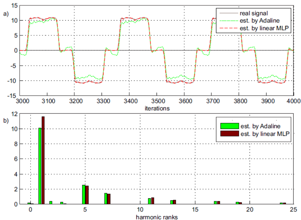
Figure 4.3 Estimation of the harmonic terms of a current from a real nonlinear load with a linear MLP and an ADALINE. a) Real and constructed signals b) Estimated spectrum histograms
