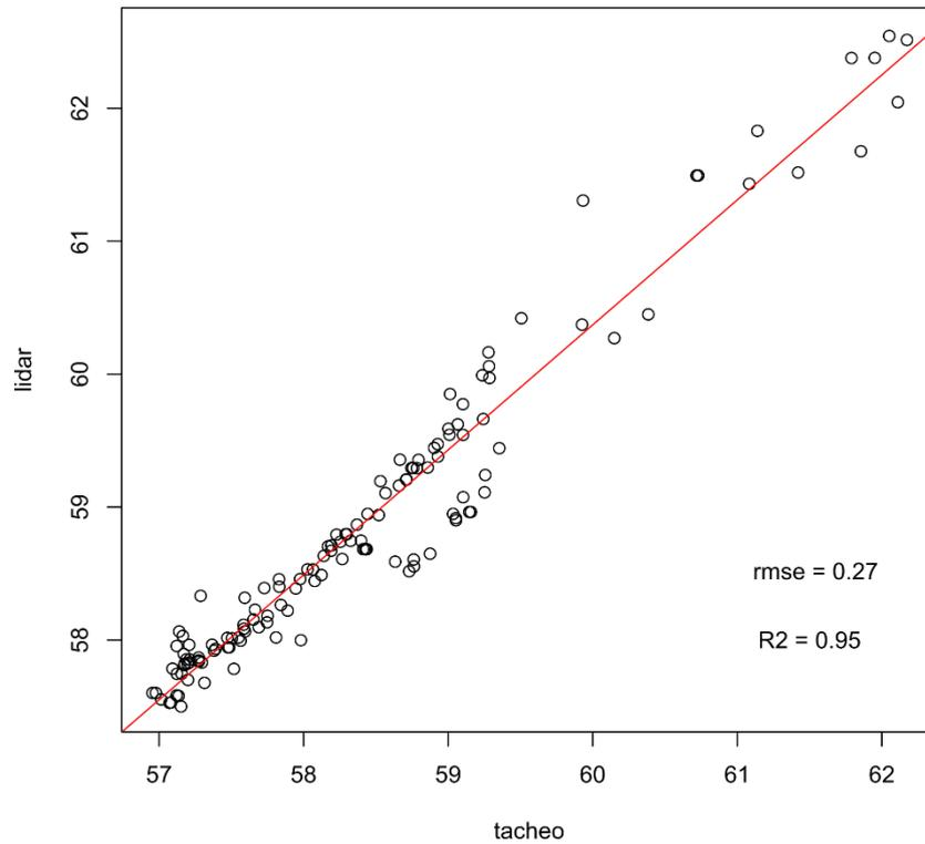
Figure 6-2: correlation between DEM and Tachometer elevation
