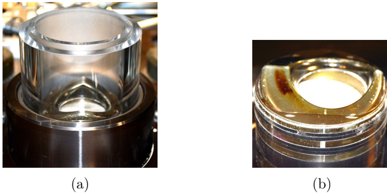
Figure 5.1: (a) Transparent quartz cylinder, (b) Piston crown.
