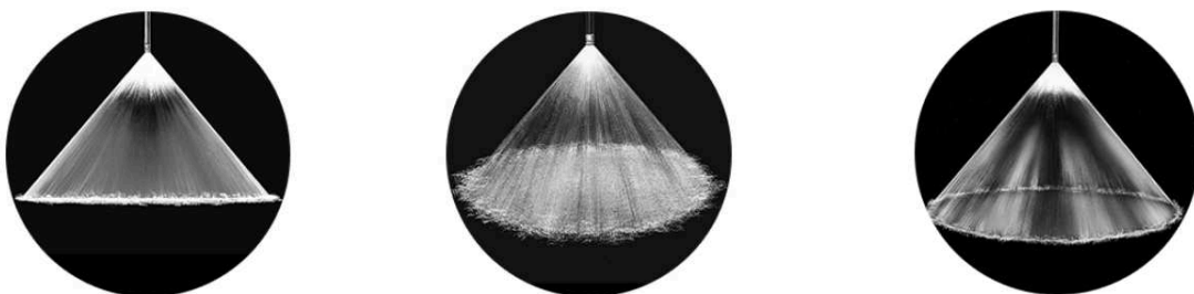
Figure 5.16: Basic spray patterns. Flat fan (left), full cone (middle), and hollow cone nozzle (right) [22].
