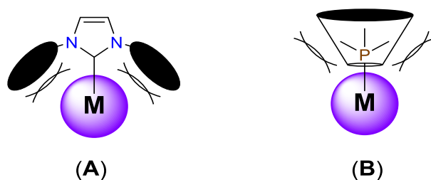
Figure 8. Models of NHC ( A ) and phosphine ( B ) ligands' steric impact. The N -substituents are spatially close to the metal center taking a cavity shape. Phosphine substituents point away from the metal center in a cone shape.
