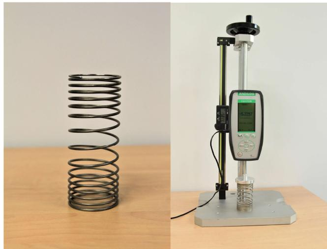
Figure 3.7: Manufactured variable pitch spring and measuring equipment
