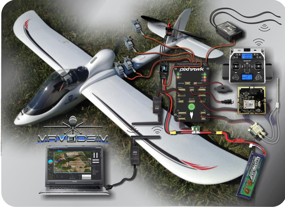
Experimental platform with the Pixhawk autopilot and used electronics.
