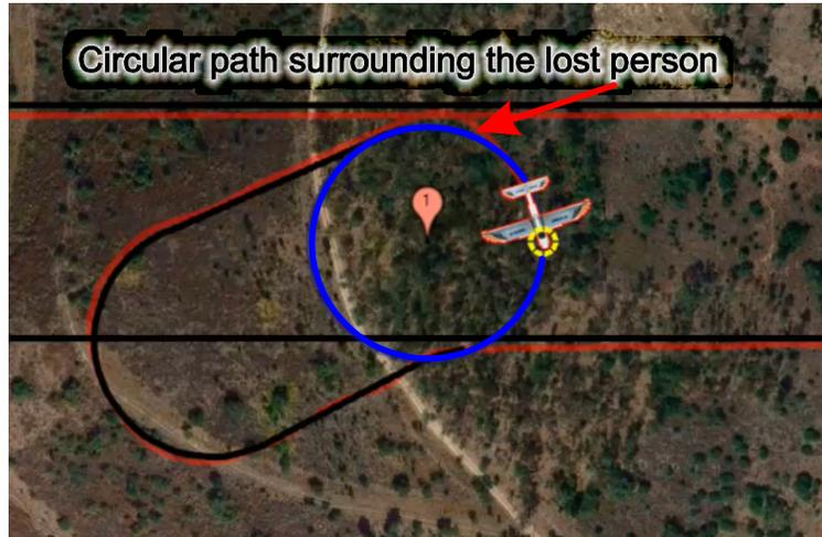
Figure 4-1: Circular path generated to surround the missing person.
