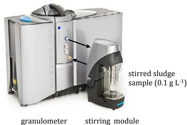
Figure II.17. Schematization of the experimental setup for the particle size analysis using the granulometer.
