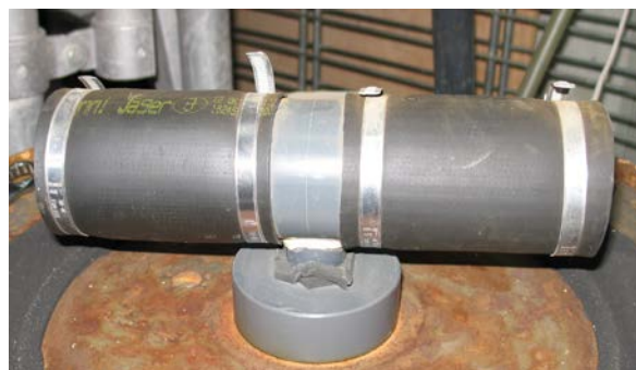
Figure II.2 Fine bubble diffuser used in the oxygen transfer tests
