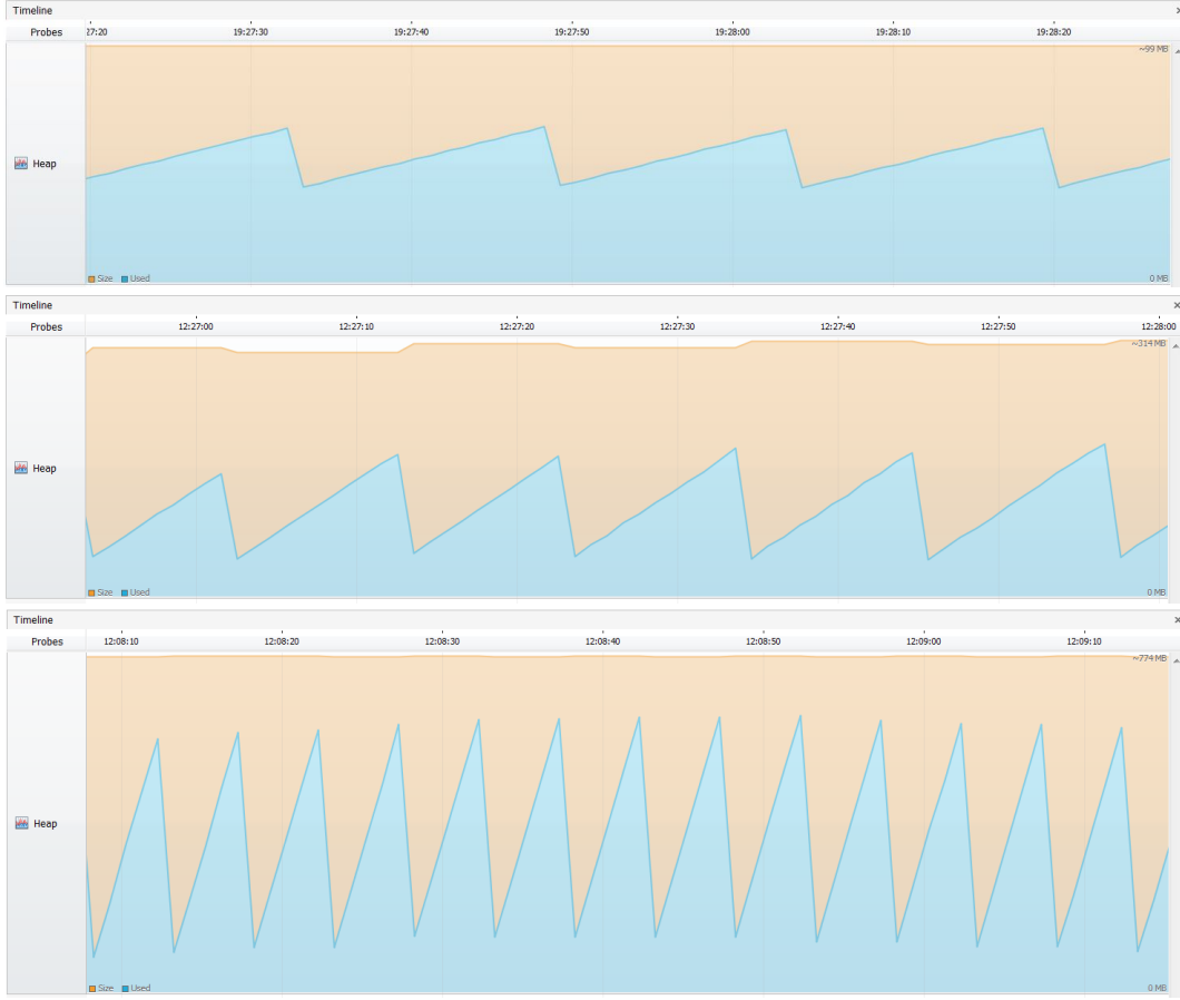
Figure 5.3.: The real-time monitoring of memory consumption of Q_1
