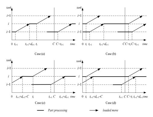
Figure 5.3 Four types of tank states for the time window constraints.
