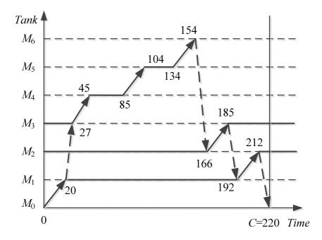
Figure 4.9 Hoist move sequence 0-3-4-5-2-1 with C=220.
