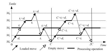
Figure 3.1 An example of cyclic scheduling problem with a single hoist. According to the notation in (Manier and Bloch, 2003) dedicated to hoist
