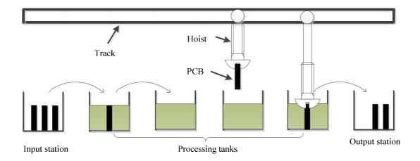
Figure 1.1 A typical automated PCB electroplating line with two hoists.
