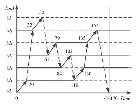
Figure 4.7 Hoist move sequence 0-5-3-2-1-4 with C=170.
