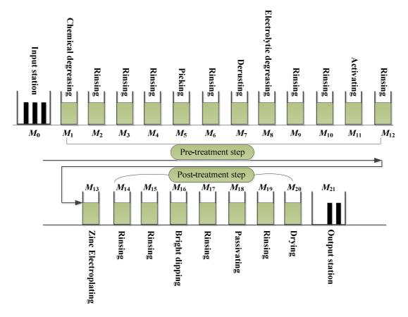
Figure 4.10 Zinc electroplating process for the selected problem.
