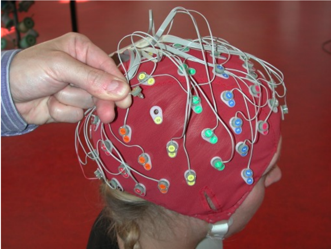
Fig. 1.4 EEG Cap is used to read the EEG signals
