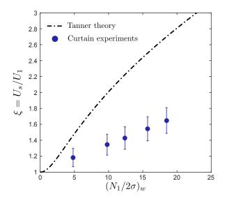
Figure 4.13 – Comparison between the experimental die swell ratio  $\xi = U_s/U_1$  for the data of figure 4.4 and the values predicted by Tanner's unconstrained recovery theory (equation 4.18) where we use  $(N_1)_w = N_1(\dot{\gamma}_w) = \Psi \dot{\gamma}_w^{\alpha_1}$  and  $(\sigma)_w = \sigma(\dot{\gamma}_w) = K_0 \dot{\gamma}_w^n$  where  $\dot{\gamma}_w$  is the wall shear rate (equation 4.19). Since  $N_1 \propto \sigma^m$ , we use  $m = \alpha_1/n$ .
