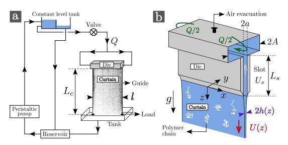
Figure 3.2 – Schematic of the hydraulic loop (a) and of the slot die (b).
