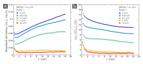
Figure 5.8 – (a) Time-averaged standard deviation  $\langle \sigma_U \rangle_t$  (equation 5.4) against z for the HPAM solutions of table B.5. (b): Relative modulation amplitude  $\langle \sigma_U / \langle U \rangle_x \rangle_t$  for the same liquids. The curtain length is  $L_c = 30$  cm
