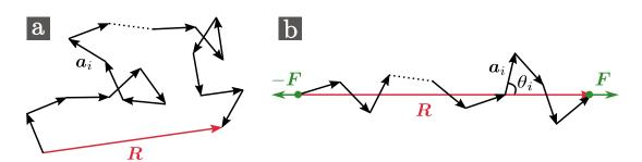
Figure 2.8 – Ideal chain.  $\mathbf{R}$  is the end-to-end vector and  $\mathbf{a}_i$  are the Kuhn vectors. (a): unconstrained (random walk at equilibrium) and (b): constrained by a force  $\mathbf{F}$ , each Kuhn segment  $\mathbf{a}_i$  makes and angle  $\theta_i$  with the force direction.
