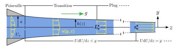
Figure 1.1 – Sketch of an infinitely long Newtonian curtain (cross-sectional view). The local vertical velocity field u(y, z) switches from a Poiseuille flow inside the slot to a plug flow at a distance  $z = L_v^*$  from the slot. In parallel, the mean velocity field U(z) averaged over the curtain thickness is characterised by a transition from a sub-gravitational regime to an asymptotic free-fall regime at a distance  $z = z_v^*$  from the slot.
