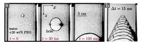
Figure 5.1 – Time evolution of a hole forming spontaneously in a curtain of 20 wt% PEG solvent with flow rate  $q = 3.3 \text{ cm}^2/\text{s}$  and length  $L_c = 30 \text{ cm}$ . The hole is advected by the flow (self-healing). (b): Image superposition.
