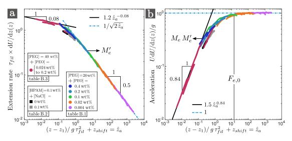
Figure 4.12 – (a) Dimensionless extension rate  $\tau_{fil} dU/dz(z)$  and (b) dimensionless acceleration U dU/dz(z)/g versus  $(z - z_1)/z_e + z_{shift}$  for the curtains of figure 4.11. The master curve  $M_e$  reaches the asymptotic free-fall regime at  $z/z_e$  about  $F_{e,0} = 12 \pm 5$  since  $M_e M'_e(F_{e,0}) = 0.95$ , where 0.95 is an arbitrary value close to 1.
