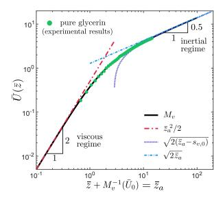
Figure 4.10 – Superposition of the experimental velocity field of the pure glycerin curtain of figure 4.1 ( $\overline{U}_0 = 0.14$ ) and of the Newtonian master curve shown previously in figure 1.3.b. The master curve  $M_v$  is characterised by an initial sub-gravitational viscous regime and an asymptotic free-fall regime (equation 1.25).
