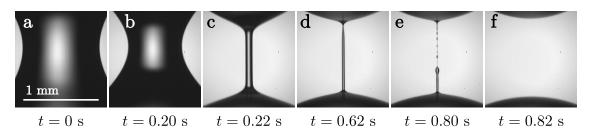
Figure 3.8 – Different stages of the thinning process of a filament made of a 0.01 wt% PEO solution with 20 wt% PEG solvent (raw images).
