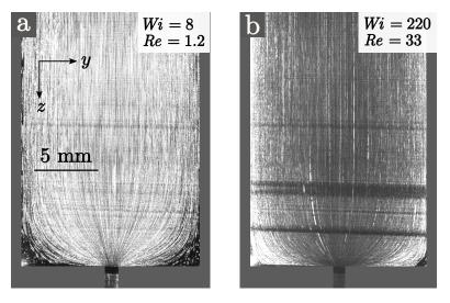
Figure 6.6 – Side view of the flow pattern for solution P2 extruded at the lowest flow rate (a)  $q = 0.42 \text{ cm}^2/\text{s}$  and the largest flow rate (b)  $q = 11 \text{ cm}^2/\text{s}$ . The respective Weissenberg and Reynolds numbers are shown. These images are obtained by superposition of successive images.
