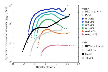
Figure 3.10 – Apparent extensional viscosity  $\eta_{app}$  (equation 3.19) as a function of the Hencky strain  $\epsilon$  (equation 3.10) for PEO solutions with 20 wt% PEG solvent and for HPAM solutions at  $T = 20^{\circ}$ C.
