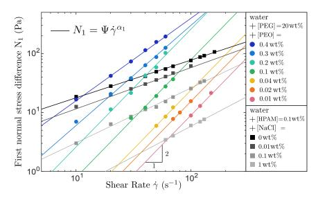
Figure 3.6 – First normal stress difference  $N_1(\dot{\gamma})$  for PEO solutions with 20 wt% PEG solvent and for HPAM solutions at  $T = 20^{\circ}$ C. Data are fitted with a power law (equation 3.8).
