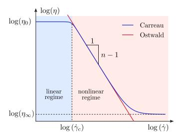
Figure 2.4 – Apparent viscosity  $\eta$  against shear rate  $\dot{\gamma}$  according to Carreau 2.41 and Oswald 2.42 laws. The boundary between the linear and nonlinear regime is  $\dot{\gamma} = \dot{\gamma}_c$ .
