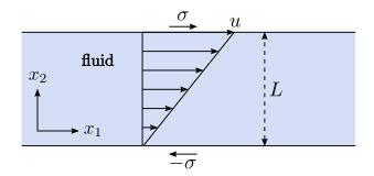
Figure 2.2 – Shear flow of a viscous fluid between two parallel plates separated by a distance d, one moving at velocity u and the other one stationary (Couette flow).
