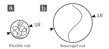
Figure 2.7 – Flexible ((a),  $\chi \gg 1$ ) and semi-rigid ((b),  $\chi \ge 1$ ) polymer chain.
