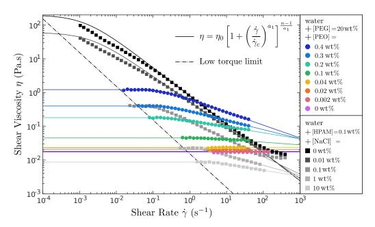
Figure 3.5 – Shear viscosity  $\eta(\dot{\gamma})$  for PEO solutions with 20 wt% PEG solvent and for HPAM solutions at  $T = 20^{\circ}$ C. Data are fitted with a Carreau law (equation 3.7). The low-torque limit is shown.
