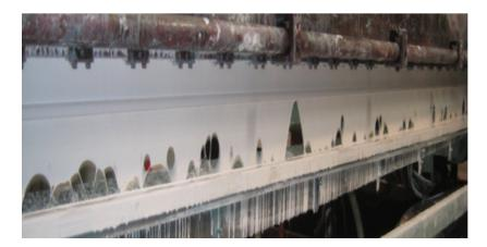
Figure 1.5 – Industrial curtain used in curtain coating (the liquid is a paint). Photo taken by Julien Beaumont from Saint Gobain Recherche in 2015 in Avilés.
