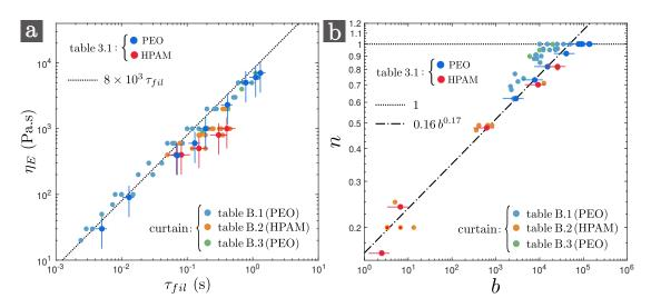
Figure 3.12 – Graphic representation of some of the rheological parameters of table 3.1 plus the rheological parameters of the solutions used in curtain experiments (see tables B.1, B.2 and B.3). (a): Terminal extensional viscosity  $\eta_E$  versus the extensional relaxation time  $\tau_{fil}$ . (b): Degree of shear-thinning *n* versus the effective flexibility parameter *b*.
