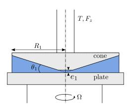
Figure 3.4 – Schematic representation of a cone-plate shear rheometer.
