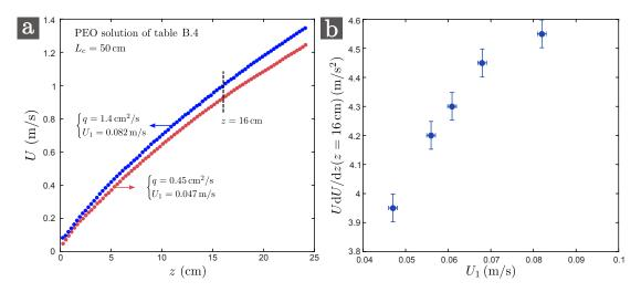
Figure 4.6 – (a): Velocity field U(z) for the PEO solution of table B.4 extruded at flow rates  $q = 0.45 \text{ cm}^2/\text{s}$  and 1.4 cm<sup>2</sup>/s. The liquid velocity  $U_1$  at  $z_1 \approx 2.5$  mm from the slot is respectively 0.047 m/s and 0.082 m/s. (b): Local acceleration UdU/dz at an arbitrary distance z = 16 cm from the slot versus initial velocity  $U_1$ . The curtain length is  $L_c = 50$  cm.
