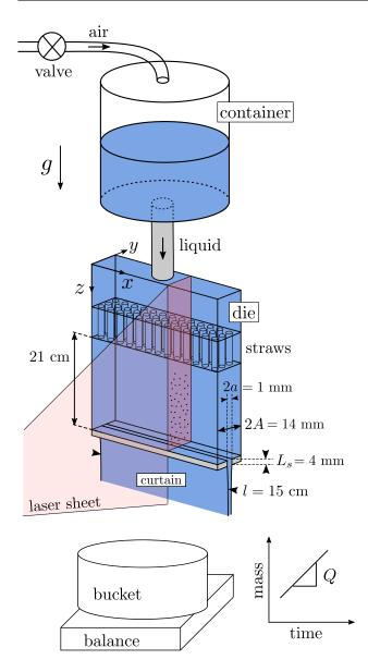
Figure 6.3 – Experimental set-up for visualisations of the flow structure upstream of the slot. The flow is illuminated by a laser sheet. We visualise the flow along two different planes: a z-y plane situated at a few centimetres from the side wall (side view, shown in this figure) and the z-x plane situated along the slot (y = 0) which is the plane of symmetry of the die (front view).
