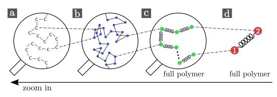
Figure 2.6 – Successive approximations of a polymer chain from the monomer scale (a) to the Kuhn length scale (b) where polymer molecules are modelled bead-rod chains, and from the bead-spring chain model (c) to the elastic dumbbell model (d).
