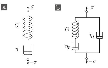
Figure 2.3 – (a) Maxwell model: purely viscous damper of viscosity  $\eta$  in serie with a purely elastic spring of elastic modulus G. (b) Jeffrey model: Maxwellian spring-damper element of elastic modulus G and viscosity  $\eta_p$  (polymers) in parallel with a purely viscous damper of viscosity  $\eta_s$  (solvent).
