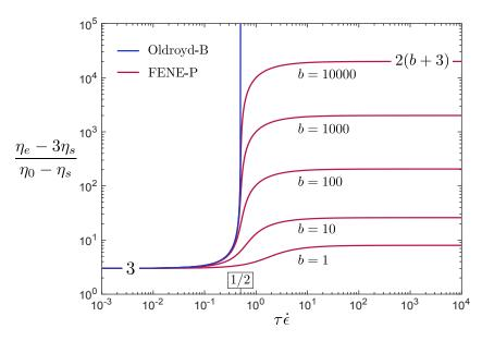
Figure 2.5 – Dimensionless polymer contribution to the extensional viscosity  $\eta_e$  (asymptotic value  $t \to +\infty$ ) versus dimensionless extension rate  $\tau \dot{\epsilon}$  for the Oldroyd-B (equation 2.39) model and the FENE-P (equation 2.51) model for different values of b.
