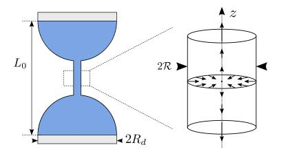
Figure 3.7 – Schematic representation of a thinning cylindrical filament.
