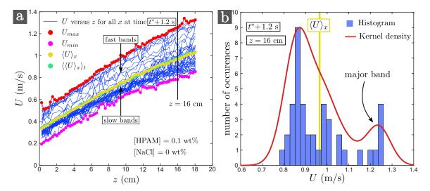
Figure 5.6 – Same as figure 5.5 but 1.2 seconds later. The velocity field (a) and the histogram (b) show the appearance of a band of fluid which is much faster than the others ("major band") and which can clearly be identified in the curtain movie.
