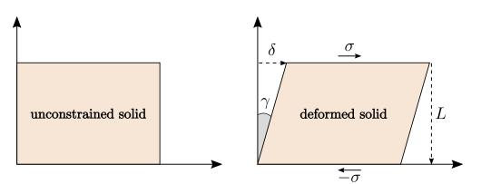
Figure 2.1 – Shear deformation of magnitude  $\gamma = \delta/L$  of an elastic solid.
