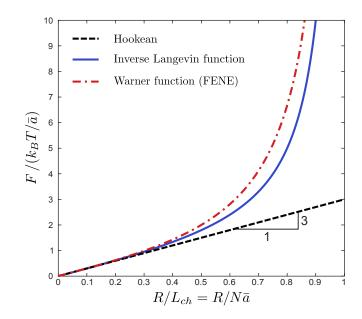
Figure 2.9 – Comparison between the Hookean function (equation 2.58), inverse Langevin function (equation 2.59) and Warner (FENE) function for the magnitude F of the polymer restoring force.
