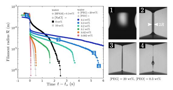
Figure 3.9 – Left: minimum filament radius  $\mathcal{R}$  as a function of time  $t - t_s$  where  $t_s$  marks the transition to the elasto-capillary (exponential) regime for PEO solutions with 20 wt% PEG solvent and for HPAM solutions at  $T = 20^{\circ}$ C. Right: Four images of a filament of a 0.2 wt% PEO solution during the thinning process. These four steps are reported on the corresponding  $\mathcal{R}(t)$  curve on the left.
