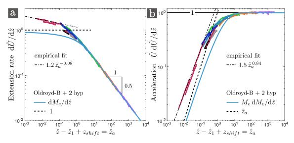
Figure 4.18 – Extension rate  $dM_e/d\hat{z}$  (a) and acceleration  $M_e dM_e/d\hat{z}$  (b) for the master curve  $M_e$  of figure 4.17.b, compared respectively with the experimental data of figure 4.12.a and 4.12.b.
