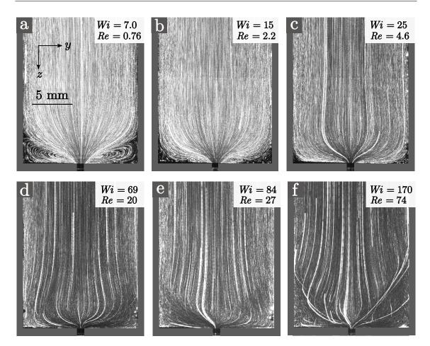
Figure 6.7 – Side view of the flow pattern for solution P3 extruded at flow rates  $q = 0.40 \text{ cm}^2/\text{s}$  (a),  $q = 0.83 \text{ cm}^2/\text{s}$  (b),  $q = 1.4 \text{ cm}^2/\text{s}$  (c),  $q = 3.9 \text{ cm}^2/\text{s}$  (d),  $q = 4.8 \text{ cm}^2/\text{s}$  (e),  $q = 9.8 \text{ cm}^2/\text{s}$  (f). The respective Weissenberg and Reynolds numbers are shown. These images are obtained by superposition of successive images.
