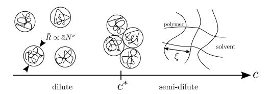
Figure 2.10 – Boundary between the dilute and semidilute regime for polymer solutions. In the semidilute regime, polymer chains are entangled and  $\bar{\xi}$  is the average distance along a chain between two contacts with other chains.
