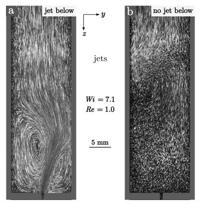
Figure 6.8 – Side view of the flow pattern for solution H1 extruded at flow rate  $q = 0.27 \text{ cm}^2/\text{s} < q_{min}$  where the x position of the laser sheet matches (a) or does not match (b) the position of a jet below the slot. The respective Weissenberg and Reynolds numbers are shown. These images are obtained by superposition of successive images.
