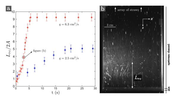
Figure 6.12 – (a): Time evolution of the dimensionless size  $L_{rc}/2A$  of the perturbed recirculation area when initiating a sudden flow of flow rate  $q = 2.5 \text{ cm}^2/\text{s}$  (Wi = 67 and Re = 14) and  $q = 6.3 \text{ cm}^2/\text{s}$  (Wi = 160 and Re = 34) for the solution H1. (b): Example of flow pattern during the transient rising of the perturbed recirculation area for  $q = 6.3 \text{ cm}^2/\text{s}$  at a time reported in figure (a).
