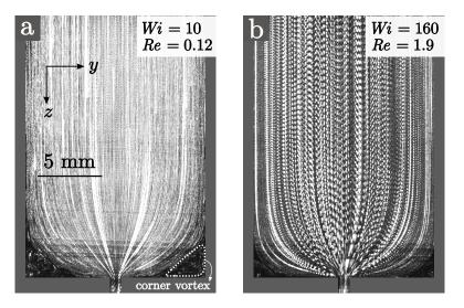
Figure 6.5 – Side view of the flow pattern for solution P1 extruded at the lowest flow rate (a)  $q = 0.29 \text{ cm}^2/\text{s}$  and the largest flow rate (b)  $q = 4.7 \text{ cm}^2/\text{s}$ . The respective Weissenberg and Reynolds numbers are shown. These images are obtained by superposition of successive images.
