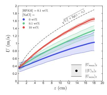
Figure 5.7 – Amplitude of the velocity distribution for three 0.1 wt% HPAM solutions with different salt concentrations (see table B.5). The average velocity  $\langle \langle U \rangle_x \rangle_t$  is compared to the time averages or the  $\langle U_{min} \rangle_t$  and  $\langle U_{max} \rangle_t$  of the minimum and maximum velocities  $U_{min}$  and  $U_{max}$  defined in figures 5.5.a and 5.6.a. The curtain length is  $L_c = 30$  cm
