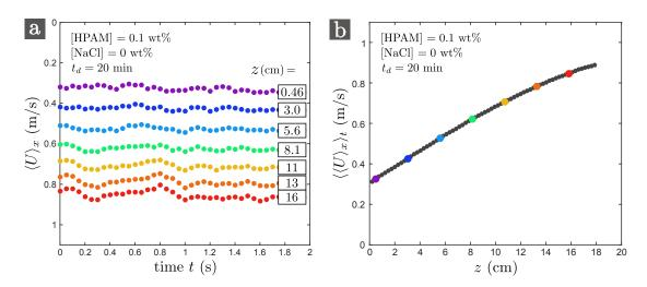
Figure 4.3 – (a): Velocity  $\langle U \rangle_x$  averaged over x versus time t (for a two seconds PIV movie) and at different distances z from the slot. Time t = 0 s corresponds to the data of figure 4.2.b. (b): Velocity  $\langle \langle U \rangle_x \rangle_t$  averaged over x and t versus z. The big coloured dots correspond to the values of figure a.
