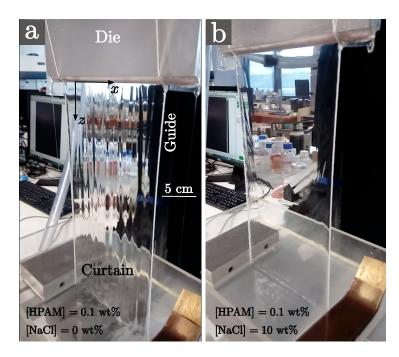
Figure 5.4 – Modulated (a) and smooth (b) curtains observed when extruding an unsalted (a) and a salted (b, [NaCl] = 10 wt% ) 0.1 wt%HPAM solution (see table B.5). In (a), the curtain organises in a succession of vertical thick and thin bands where the liquid is respectively faster and slower than average.
