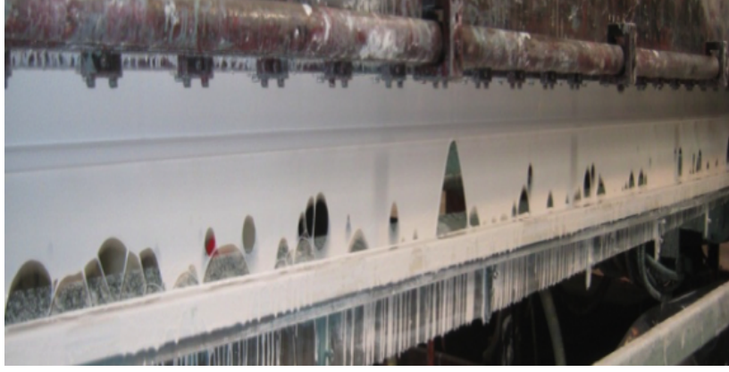
Figure 1.5 – Industrial curtain used in curtain coating (the liquid is a paint). Photo taken by Julien Beaumont from Saint Gobain Recherche in 2015 in Avilès.
