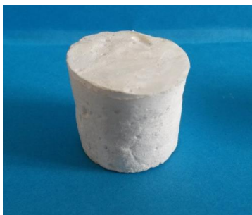
Figure 4-5. Optical photography of fully dried monolith M24 after PCM-extraction.
