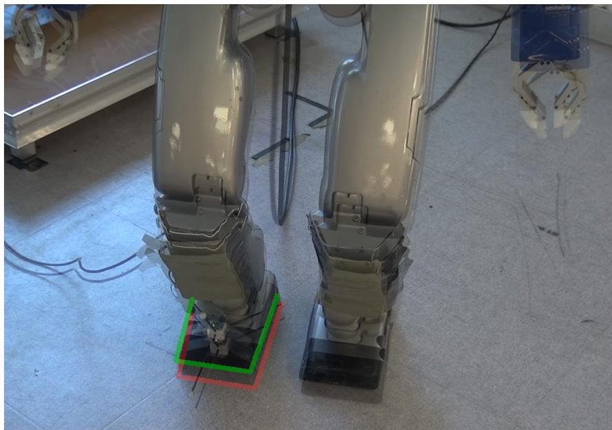
Figure 3.15: HRP2 drifts during the 'walk in place' test. We can notice the difference in both position and orientation between the **initial** and **final** poses after performing 5 steps with both right and left feet. The position drift is higher than the orientation one.
