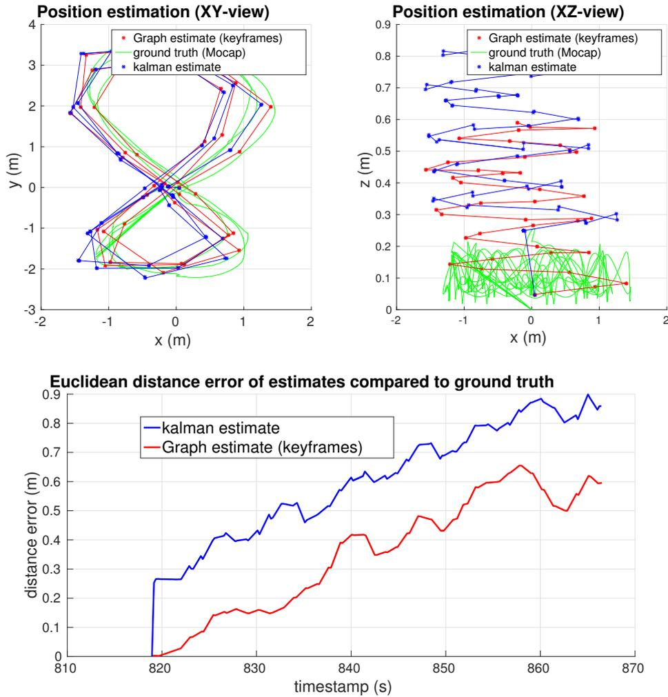
Figure 3.8: **Top:** trajectory estimation during human 8-shaped walking phases with an IMU attached to a foot. Stars in blue and red colours are respectively the reference estimated states provided in the dataset and the estimation with our approach. The continuous green line is the ground truth as given by the motion capture system. **Bottom:** Evolution of Euclidean distance errors between estimates and the ground truth for this 8-shaped walking trajectory.
