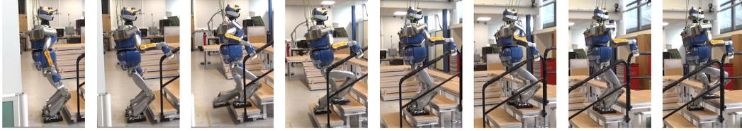
Figure 5.2: Snapshots of the climbing up 15-cm high steps motion with the HRP-2 using the stair railing.
