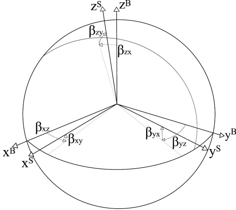
Figure 2.3: Representation of the misalignment and non-orthogonality of accelerometer and gyroscope axes in an IMU [Tedraldi 2013]. The 3D frame formed by the set of axes  $(x^B, y^B, z^B)$  is orthogonal while the frame formed by the axes  $(x^S, y^S, z^S)$  is misaligned and non-orthogonal.
