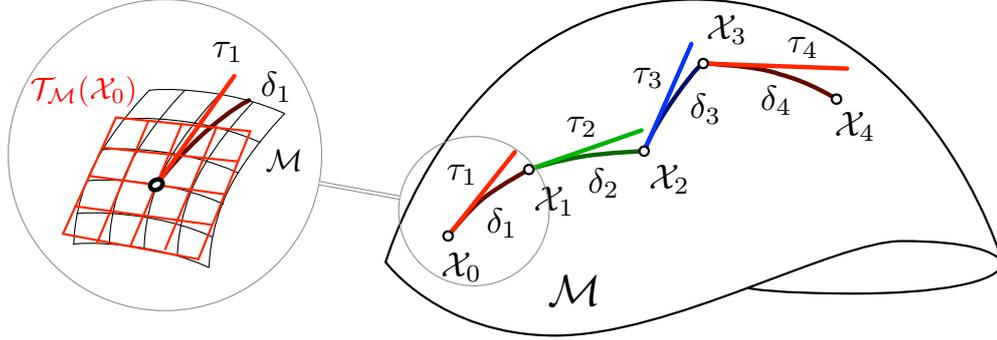
Figure 4.6: Motion integration on a manifold. Each motion data produces a step  $\tau_k \in \mathcal{T}_M(\mathcal{X}_{k-1})$ , which is retracted to a local motion increment or ‘delta’  $\delta_k \in \mathcal{M}$ , and then composed with  $\mathcal{X}_{k-1}$  to yield  $\mathcal{X}_k = \mathcal{X}_{k-1} \circ \text{retr}(\tau_k) = \mathcal{X}_{k-1} \circ \delta_k \in \mathcal{M}$ .
