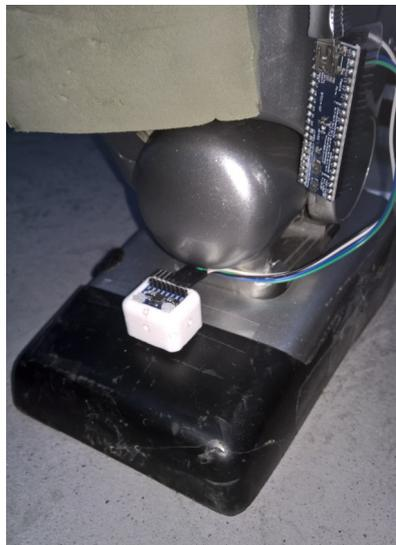
Figure 3.12: The IMU (in a white 3D-printed case) is fixed to the foot and connected to the STM32 microcontroller by I2C.
