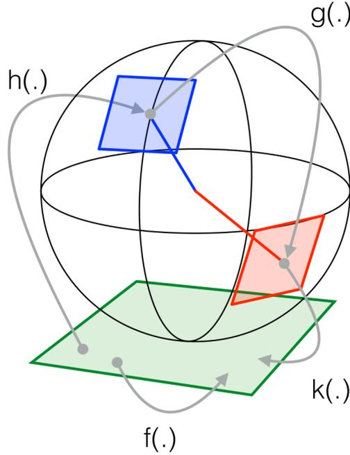
Figure C.2: Representation of the derivatives operation. We consider a situation so that variable can be either in the  $\mathbb{R}^n$  or in one of the manifolds (blue and red spaces). Then we define the functions  $f : \mathbb{R}^m \rightarrow \mathbb{R}^n$ ,  $g : S^3 \rightarrow S^3$ ,  $h : \mathbb{R}^m \rightarrow S^3$  and  $k : S^3 \rightarrow \mathbb{R}^n$ .
