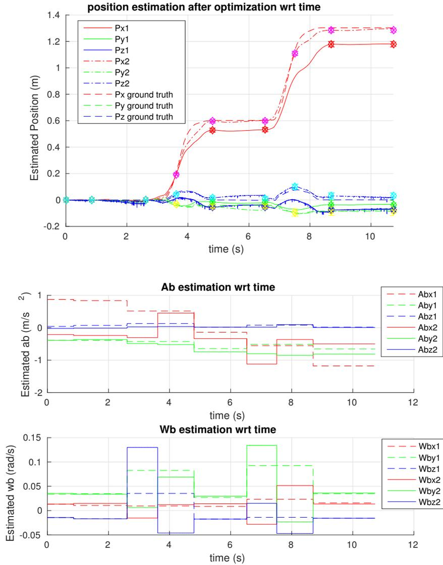
Figure 3.10: **Top**: trajectory estimation during human walking with an IMU attached to a foot. Continuous, dashed and dashed-dot lines are respectively: ground truth, estimation with zero velocity constraints only, estimation using zero velocity constraints and 1 odometry measurement during foot’s flying phase. Odometry was here built from motion capture data. **Bottom**: Evolution of corresponding estimated IMU biases
