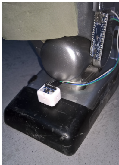
Figure 3.12: The IMU (in a white 3D-printed case) is fixed to the foot and connected to the STM32 microcontroller by I2C.
