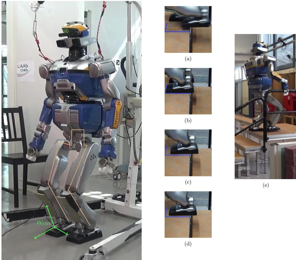
Figure 3.1: The flying foot trajectory is reconstructed through an IMU set on the foot (in green), and by fusing the information coming from the kinematic chain from the support foot to the flying one (in light brown). In the middle images (a)-(d) shows slippage while performing a multicontacts motion depicted on the right (e) (from [Carpentier 2016]).
