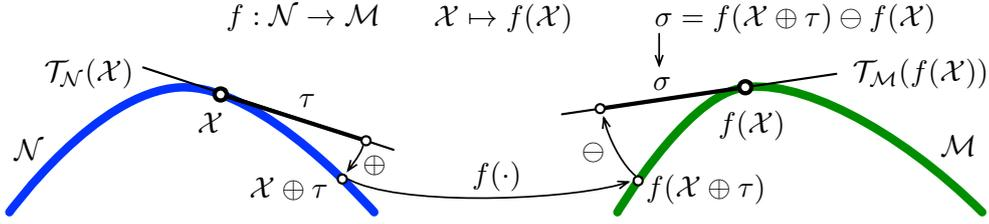
Figure 4.5: Derivative of functions acting between two manifolds  $\mathcal{N}$  and  $\mathcal{M}$ . The perturbation  $\tau \in \mathcal{T}_{\mathcal{N}}$  around  $\mathcal{X} \in \mathcal{N}$  is propagated to a perturbation  $\sigma \in \mathcal{T}_{\mathcal{M}}$  around  $f(\mathcal{X}) \in \mathcal{M}$  through the processes of plus, apply  $f()$ , and minus (arrows). The derivative is simply  $\lim_{\tau \rightarrow 0} \sigma/\tau$ .
