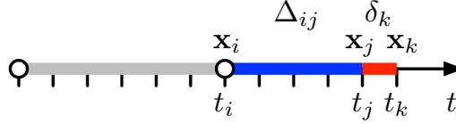
Figure 4.8: The pre-integrated delta  $\Delta_{ij} \in \mathcal{D}$  contains all motion from the last KF at time  $i$ , up to time  $j$ , so that  $\mathbf{x}_j = \mathbf{x}_i \boxplus \Delta_{ij}$ . The current delta  $\delta_k \in \mathcal{D}$  contains the motion from times  $j$  to  $k$ , computed from the last motion measurement at time  $k$ , so that  $\mathbf{x}_k = \mathbf{x}_j \boxplus \delta_k = \mathbf{x}_i \boxplus \Delta_{ij} \boxplus \delta_k = \mathbf{x}_i \boxplus \Delta_{ik}$ .
