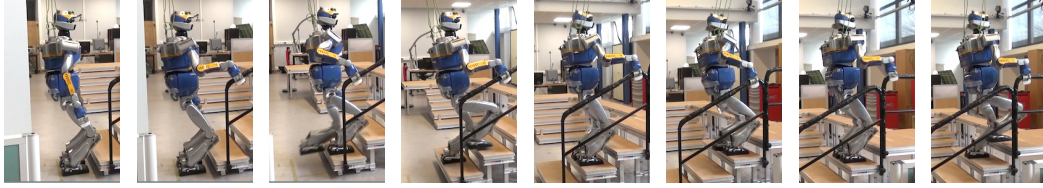
Figure 5.2: Snapshots of the climbing up 15-cm high steps motion with the HRP-2 using the stair railing.
