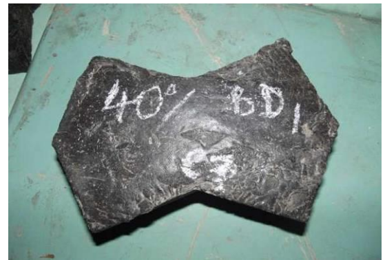
Fig. 3: Material containing 40% plastic
