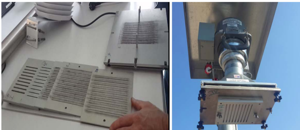
Figure 3.2: High volume air sampler and cascade impactor
