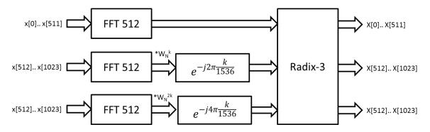
Figure 5.2 Structure of the 1536-point FFT
