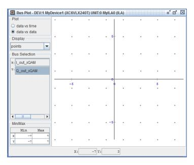
Figure 4.9 Example of baseband level verification using ChipScope Pro Analyzer for 64-QAM data.
