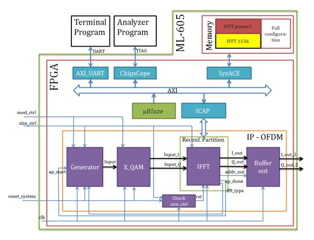
Figure 6.4 The architecture of the multi-mode FFT with hardware reconfiguration.
