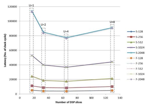
Figure 5.5 The latency vs number of DSP slices (S is for Simulation after synthesis and F is for the Formula estimate) (frequency = 100 MHz).
