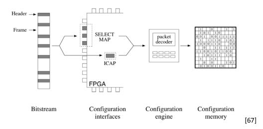
Figure 3.7 The reconfiguration chain for a Virtex FPGA.
