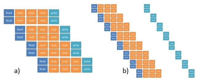
Figure 5.7 Timing chronogram of the third loop based on Algorithm 7: a) U = 4; b) U = 8.
