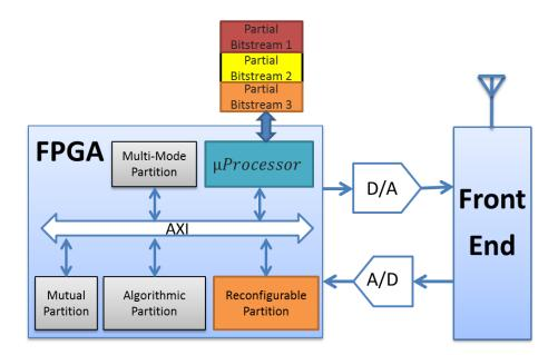
Figure 4.4 System architecture for FPGA-based SDR.
