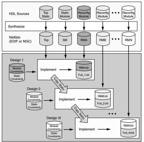
Figure 3.10 Partial reconfiguration software flow [66].
