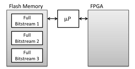
Figure 2.14 Separated configurations.
