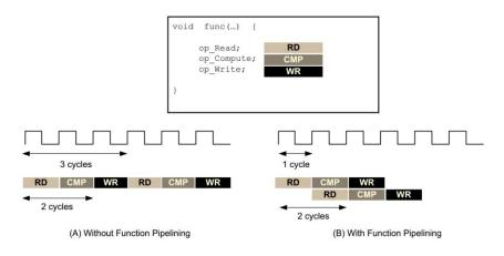
Figure 3.5 Pipeline optimization [66].
