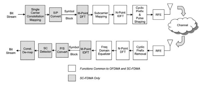
Figure 2.10 A basic SC-FDMA transmitter and receiver [29].
