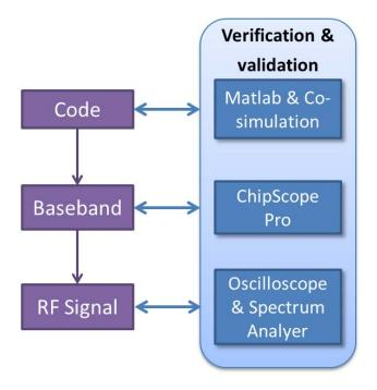
Figure 4.7 Verification and validation tools for the flexible radio design flow.
