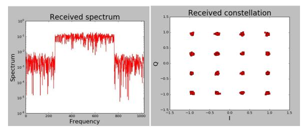
Figure 6.7 Received spectrum and 16-QAM received constellation for an AWGN channel.
