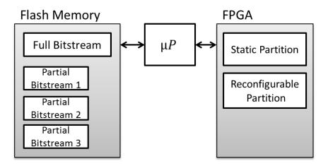
Figure 2.15 Partial reconfiguration.
