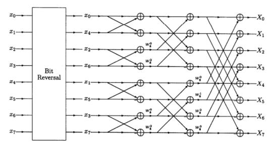
Figure 2.11 An eight-point DFT, divided in four two-point DFTs with bit reversal on inputs [33].
