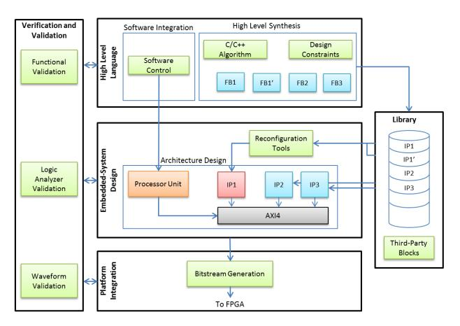
Figure 4.5 Proposed design flow for Flexible Radio using FPGA-based SDR.
