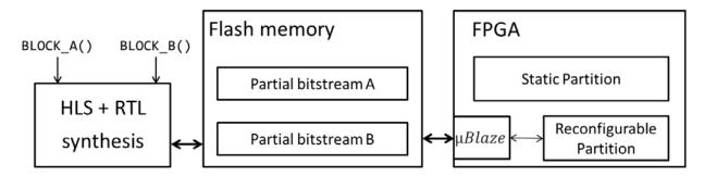
Figure 4.1 Design approach based on hardware reconfiguration.
