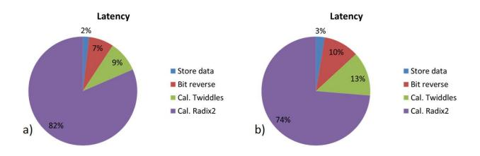
Figure 5.4 FFT latency with unrolling factor U = 1 a) FFT 2048; b) FFT 128.
