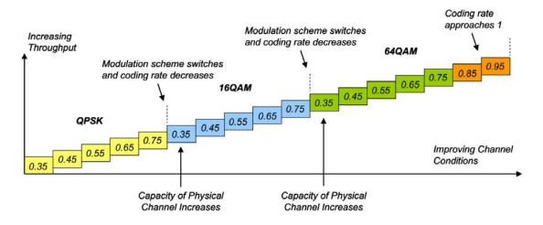
Figure 2.9 Physical layer coding rate as a function of channel conditions and modulation scheme [31].
