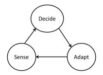
Figure 2.4 The cognitive radio's cognition cycle.
