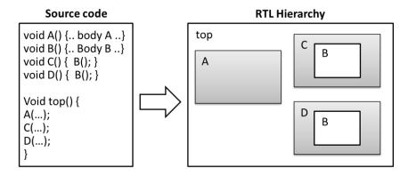
Figure 3.3 RTL hierarchy after HLS synthesis.
