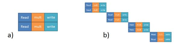
Figure 5.13 Timing chronogram of the third loop at 50 MHz: a) U = 1; b) U = 4.
