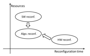
Figure 4.2 Tradeoff between resources and reconfiguration time for the different reconfigurations.
