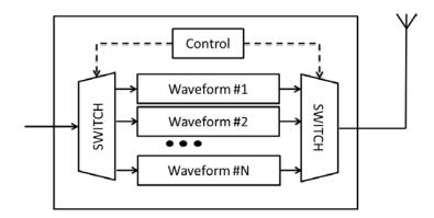
Figure 2.5 Basic software-controlled radio.
