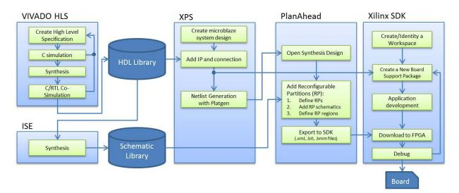
Figure 4.6 Step-by-step development flow using Xilinx tools.
