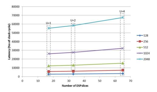
Figure 5.9 Latency vs number of DSPs at frequency 50MHz.
