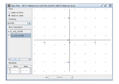
Figure 6.2 The 64-QAM constellation with ChipScope Pro.
