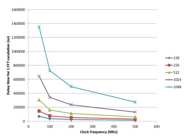
Figure 5.14 Time to compute 1 FFT vs frequency, U = 4
