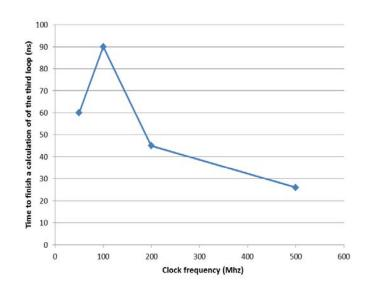
Figure 5.10 The third loop computation time vs clock frequency for U = 1 (= time to compute a radix-2 FFT)
