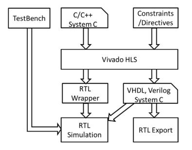
Figure 3.2 The Vivado HLS design flow.
