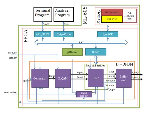
Figure 6.1 Overview of the architecture of the multi-mode FFT.
