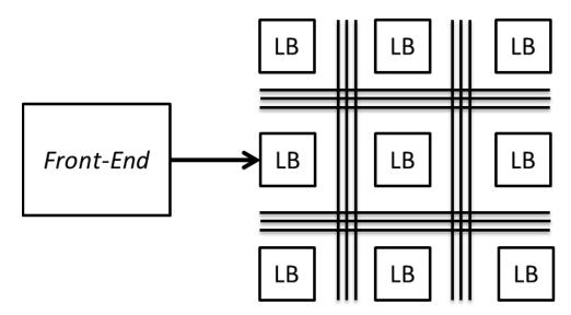
Figure 2.13 FPGA-based approach.
