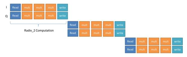
Figure 5.6 Timing chronogram of the third loop based on Algorithm 6.
