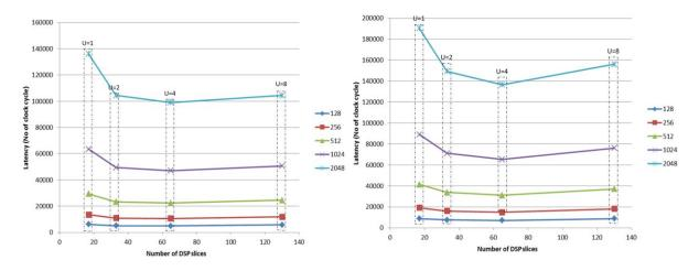
Figure 5.8 Latency vs number of DSPs for clock frequencies 200Mhz (left) and 500MHz (right).
