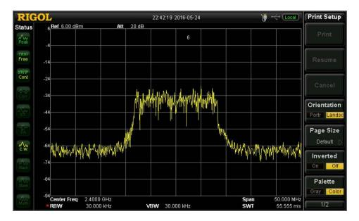
Figure 4.10 Example of RF signal analysis: an OFDM-based RF spectrum.
