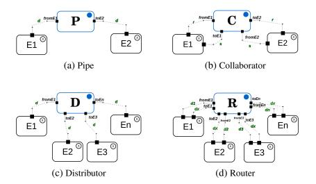
Figure 91 - Mediators types for communication
