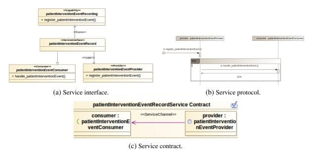
Figure 31 – Service interface, contracts and protocol diagrams for the capability *patientInterventionEventRecording*
