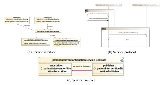
Figure 35 – Service interface, contracts and protocol diagrams for the capability *patientInterventionSituationSending*
