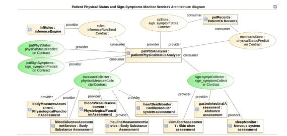
Figure 79 – Services architecture for the BPSv001-1 Patient Physical Status and Sign-Symptoms Monitor of DiaManT@Home.
