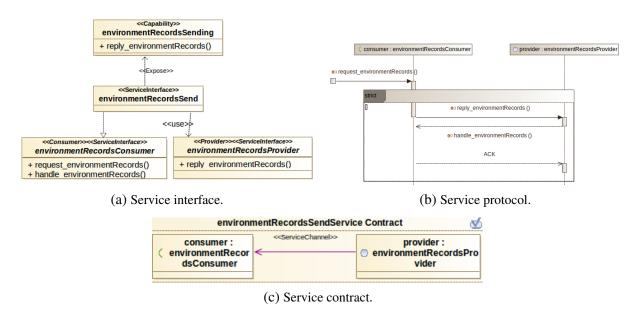
Figure 46 – Service interface, contracts and protocol diagrams for the capability *environmentRecordSend-ing*
