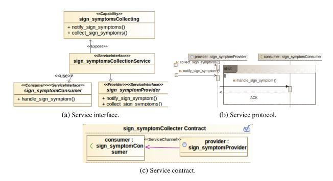
Figure 20 - Service interface, contracts and protocol diagrams for the capability sign\_symptomsCollecting
