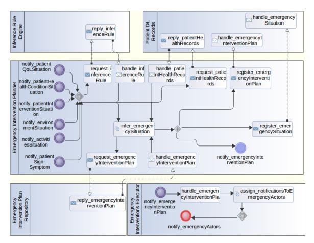
Figure 58 – Process diagram for the the business process service BPSv011 - Emergency manager.
