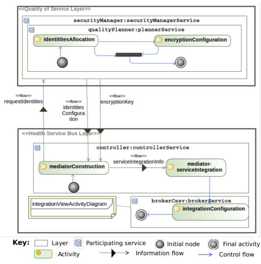
Figure 75 – Authentication diagram: assignation of service identities in *HomecARe*.
