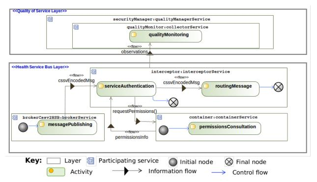
Figure 76 – Authorization diagram: verification of services permissions in HomecARe.
