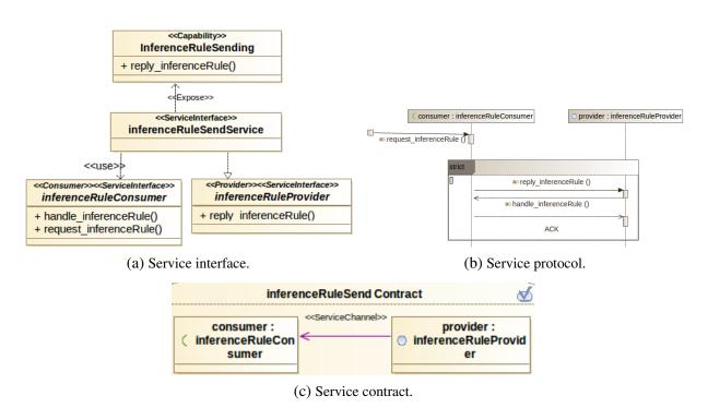
Figure 22 - Service interface, contracts and protocol diagrams for the capability inferenceRuleSending
