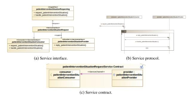
Figure 29 – Service interface, contracts and protocol diagrams for the capability *patientInterventionSituationRequesting*
