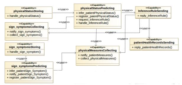
Figure 18 – Capability Diagram for the business process service BPSv001 - Patient status and sign & symptoms monitor
