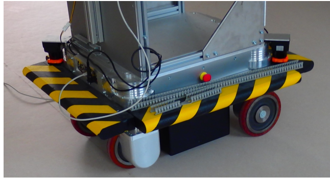
Figure 1.2: Neobotix-MPO700 steerable mobile robot used in this thesis.
