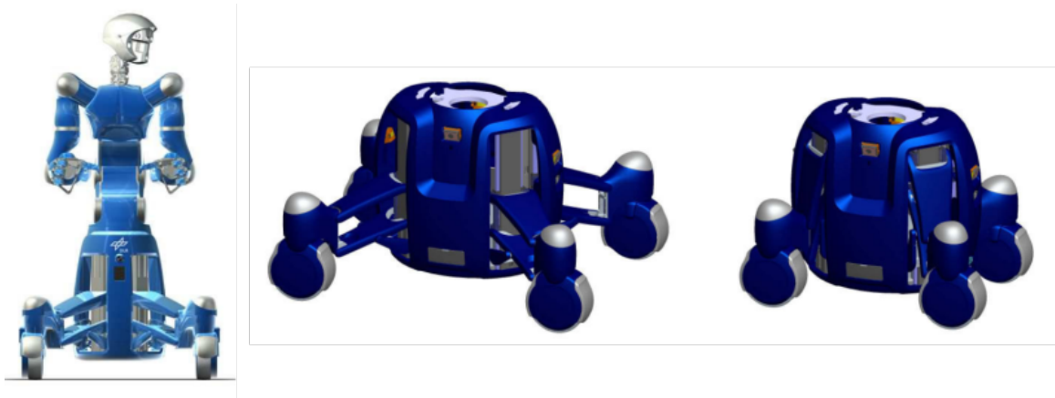
Figure 2.4: Rollin' Justin variable footprint SWMR. The dual arm mobile manipulation system [BOW + 07,FBG + 09] (left), legged SWMR extended [GFASH09] (middle) and folded (right)
