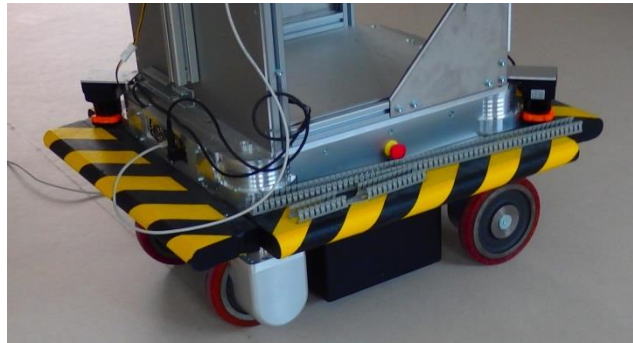
Figure 3.5: Photograph of the Neobotix MPO700 industrial SWMR.
