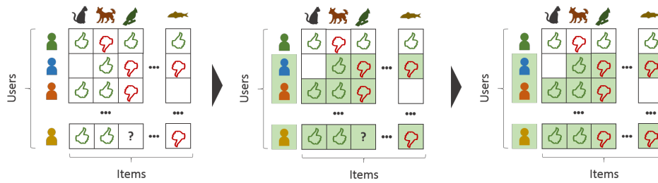
Figure 6.3.1: Example of estimation of the user’s interest in an item (pets) using collaborative filtering. The prediction is built upon the existing interactions of other users, who have similar interaction behaviour to the target user (coloured with light green).
