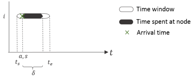
Figure 6.3.4: Illustration of parameters used in ILS. The following notations are used: a - arrival time, s - service start time, t_s - opening of the time window, t_e - closing of the time window,
